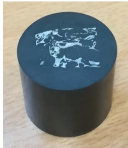
Figure 3-2. Photograph of the aluminum foam sample embedded in a conductive carbon filled resin
