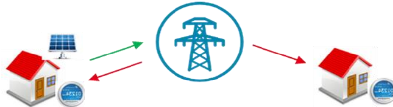
Fig. IV.9 Individual connection scheme where the Prosumer and consumer connect with grid only
