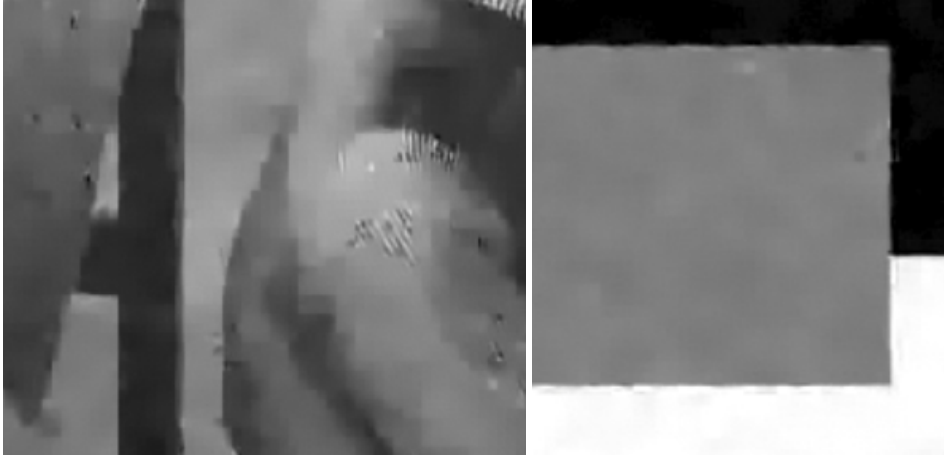
FIGURE 2.3: Issues on the reconstruction of Barbara and Cartoon with the EPLL algorithm for \sigma = 50 . We can see on the left some gray flat tints instead of the stripes. On squares, the estimation is quite accurate, with still some fluffy effect in the gray square.
