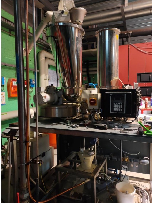
Figure III.15: Image of the feeding system: in the first sight the twin-screw feeder (K-TRON K-ML-D5-KT20), in the back, the single screw feeder and below the ejector
