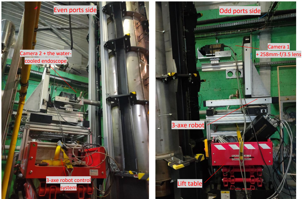
Figure III.21: The optical systems held by the 3-axe robot on the lift table from both sides of the chamber
