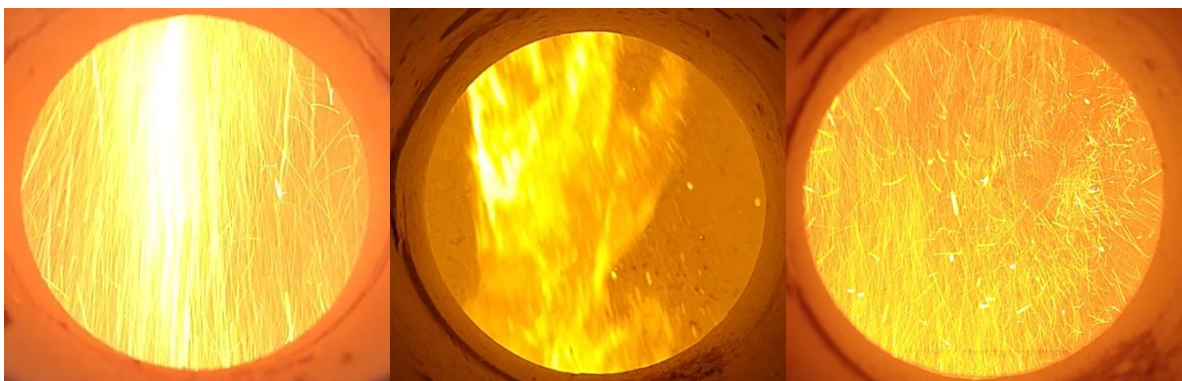
Figure VII.2: Direct images of the three pulverized biomass flames (from left to right: Pine, Pin-T and Pin-P) at port 7 (94 cm from the burner exit)
