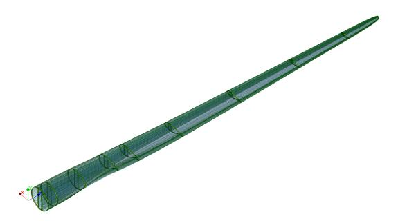
Figure 4.3: Wind turbine blade cross section in the span-wise direction equally located at the gages from FAST simulation.
