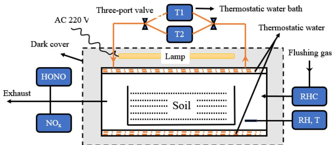
Figure 4.7 Diagram of the flow tube. RHC: relative humidity controller.
