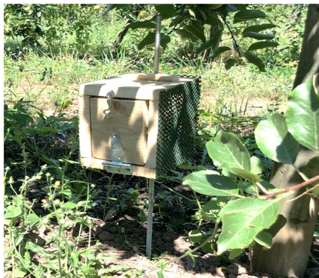
Figure 18 - Custom emergence cage. There is door in the front to introduce the pupae of M. ridens and the three other sides are covered with a plastic mesh to allow dispersal after emergence.
