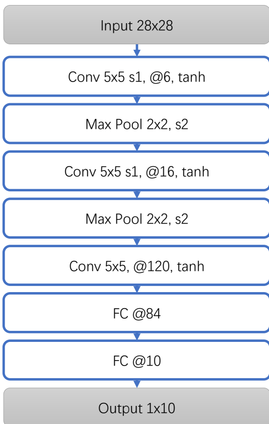
Figure 2.5: The structure of LeNet, where “Conv 5x5 s1, @6, tanh” means a convolutional layer has 6 kernels with size 5x5 and stride 1, and followed by tanh as activation function
