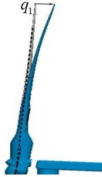
Figure 4.1 – Blade#1 flap-wise bending deflection.
