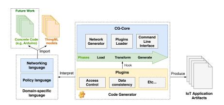
Figure 4.1 – The core components of the code generator
