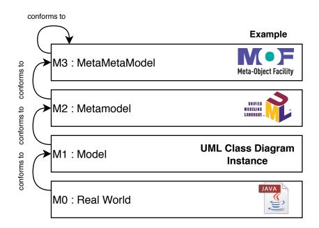
Figure 1.1 – The four-layers architecture of MDA
