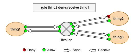
Figure 4.6 – Enforcement at the "on receive" checkpoint
