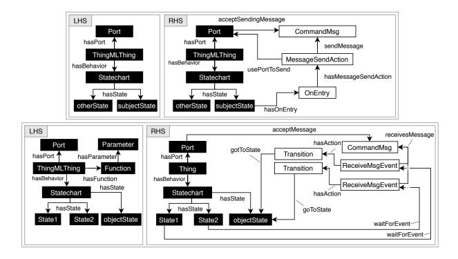
Figure 4.12 – Upper Part for Subject, Lower Part for Object; applying the trigger:goTo-State rule GTRs (4) with the subject thing having two states and the object thing having three states; white boxes are added based on the CY-Model.
