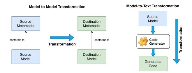
Figure 1.2 – The two types of model transformation
