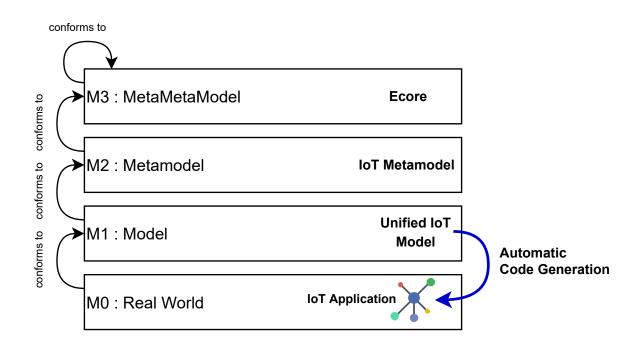
Figure 1.3 – The four-layers architecture of MDA applied to IoT
