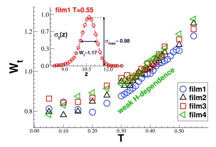
Figure 6-6: In the main panel  $W_{\rm t}(T)$  is presented for various L while the inset illustrates the determination of  $W_{\rm t}$  for film1 and T=0.55.  $\sigma_{\rm max}\approx 1$  and  $\sigma_{\rm t0}\approx 0$  in this case.
