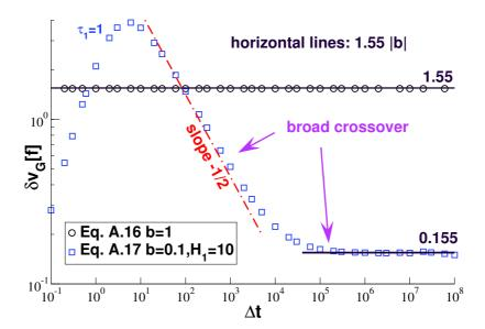
Figure A-3:  $\delta v_{\rm G}[f]$  vs.  $\Delta t$  for logarithmic creep. The circles indicate Eq. A.16 for b=1, the squares Eq. A.17 for  $H_1=10$ ,  $\tau_1=\tau_2=1$ , b=0.1 and  $\tau_3=10^{10}$  and the dash-dotted line the  $1/\sqrt{\Delta t}$ -decay of the short-time Maxwell model. The arrows emphasize the broad crossover between the Maxwell model and the plateau expected for b=0.1.
