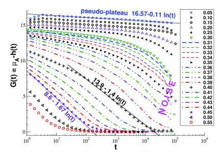
Figure 4-9: Unscaled stress relaxation modulus G(t) for film1 using half-logarithmic coordinates. G(t) increases continuously with decreasing T. For some temperatures above  $T_{\rm g}$  and for very low  $T \ll T_{\rm g}$  a logarithmic creep  $G(t) = a - b \log(t)$  is observed (thin solid lines). We shall come back to this logarithmic creep behavior in Sec. 7.4.
