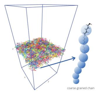
Figure 3-2: Our films consists of M = 768 coarse-grained polymer chains of length N = 16. The visualization on the left is obtained using VMD [123] for film4 with L = 49 (Sec. 3.4). The illustration on the right shows the essence of coarse-graining for a single chain where chemical details are deemed irrelevant.
