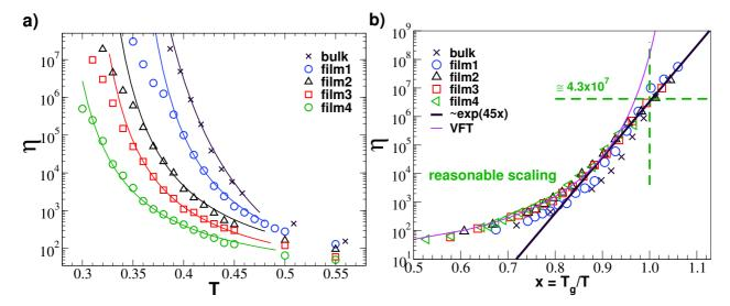
Figure 5-2: Scaling of  $\eta$  focusing on data obtained from the TTS of  $\mu(\Delta t)$  for all films and the bulk system: (a) Vogel-Fulcher-Tammann (VFT) fits (continuous lines) for  $\eta$  as a function of T. (b) Scaling of  $\eta$  as a function of  $x = T_g/T$ .
