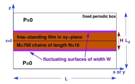
Figure 1-1: We study free-standing polymer films with M=768 oligomer chains of length N=16 monomers confined in periodic boxes with L being the imposed lateral box size in both x and y directions. The film thickness  $H \sim 1/L^2$  (to leading order) is operationally defined using the Gibbs dividing surface [57] as shown in Sec. 4.2.
