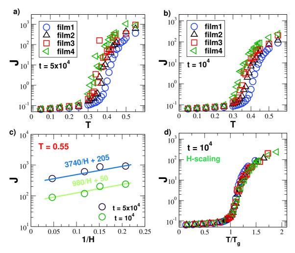
Figure 5-6: The creep compliance J(t) sampled at different times (a)  $t = 5 \times 10^4$  and (b)  $t = 10^4$  (c) Thickness dependence of J(t) also given for two different t as indicated in the figure. (d) Scaling plot for all films obtained by setting the horizontal axis  $x = T/T_g$ .
