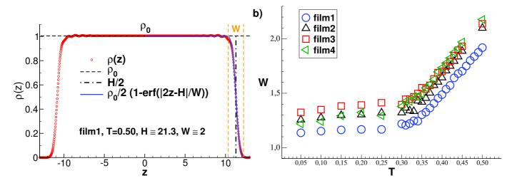
Figure 6-1: (a) Density profile  $\rho(z)$  for film1 at T=0.50. The film thickness  $H\equiv NM/\rho_0L^2$  may be obtained from the midplane density  $\rho_0$  (horizontal dashed line). Similar values are obtained by fitting the mean-field prediction given by the solid line [124]. (b) Interface width W(T) for different L.
