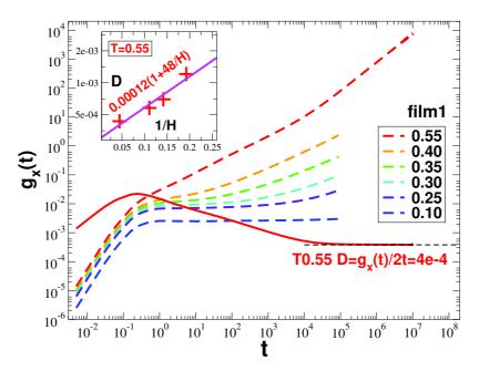
Figure 4-11: Monomer mean-square displacement (MSD)  $g_x(t)$  along the x-axis for film1 for various temperatures (dashed lines).  $g_x(t)/2t$  (solid line) is seen to converge to a diffusion constant  $D \approx 0.0004$  for the highest temperature T = 0.55. Inset: Comparison of the diffusion coefficients D for T = 0.55 for our four films demonstrating  $D \propto 1/H$  (solid line).
