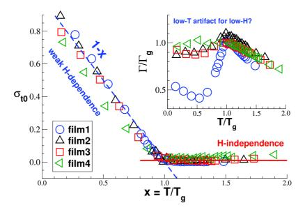
Figure 6-5: Tangential stress  $\sigma_{t0}$  at the film midplane (main panel) and surface tension  $\Gamma \equiv (\sigma_t - \sigma_{t0})H/2$  (inset) as functions of  $x = T/T_g$  for all our films. The vertical axis of the inset is made dimensionless using  $\Gamma_g \equiv \Gamma(T = T_g)$ .
