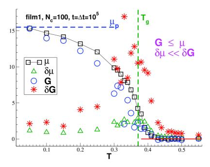
Figure 7-1: Shear modulus  $\mu$ , shear relaxation modulus G and the corresponding standard deviations  $\delta\mu$  and  $\delta G$  taken at  $t=\Delta t=\Delta t_{\rm max}=10^5$  as functions of T. The observed two inequalities  $G\leq\mu$  and  $\delta G\gg\delta\mu$  are both consequences of the stationarity relation Eq. 1.2. The corresponding error bars  $\delta\mu/\sqrt{N_c-1}$  and  $\delta G/\sqrt{N_c-1}$  are not shown.
