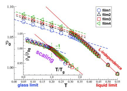
Figure 6-2: Midplane density  $\rho_0(T)$  for all our films. While  $\rho_0$  does not depend on H in the liquid limit, it decreases with increasing H in the glassy limit. This allows to determine the glass transition temperature  $T_{\rm g}$  and the midplane density  $\rho_{0\rm g} \sim 1/H_{\rm g}$  at the glass transition. Inset: Scaling of  $\rho_0/\rho_{0\rm g}$  vs  $T/T_{\rm g}$  using  $\rho_{0\rm g}$  and  $T_{\rm g}$  as indicated in Table 3.1.
