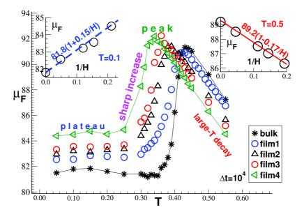
Figure 4-4: Shear-stress fluctuation  $\mu_{\rm F}$  for  $\Delta t = 10^4$ . Main panel:  $\mu_{\rm F}(T)$  for all systems. Right inset:  $\mu_{\rm F}$  decreases linearly with 1/H in the liquid limit (T=0.50). Left inset:  $\mu_{\rm F}$  increases linearly with 1/H in the solid limit (T=0.10).
