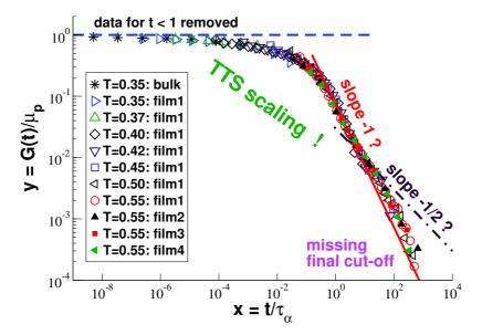
Figure 4-10: Successful TTS scaling plot of  $y = G(t)/\mu_p$  as a function of reduced time  $x = t/\tau_\alpha$  using the same relaxation times as in Fig. 4-8. The two indicated power laws (bold and dash-dotted lines) are given for comparison. Unfortunately, our production runs are too short to reveal the expected final exponential cut-off even for the highest temperatures.
