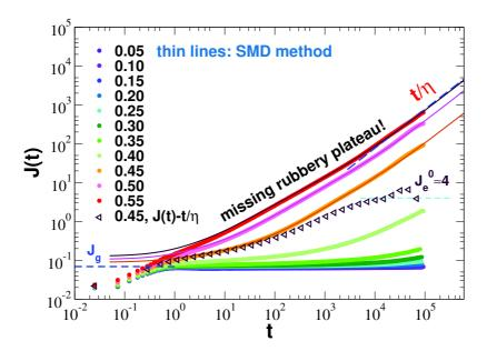
Figure 5-5: J(t) calculated using the HH (dots) and SMD (lines) methods for various temperatures. For high-T, it is also seen that the system reaches flow and  $\eta=130$  for T=0.55 is observed in the long time limit. As seen from the open triangles the same steady-state creep compliance  $J_{\rm e}^0\approx 4$  for T=0.45 is obtained as in Sec. 5.3.
