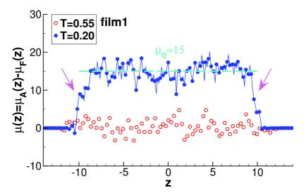
Figure 6-9: Distribution  $\mu(z) \equiv \mu_{\rm A}(z) - \mu_{\rm F}(z)$  of the shear modulus for film1 and two temperatures. While  $\mu(z)$  vanishes in the liquid limit (open circles), it becomes finite below  $T_{\rm g}$  with a plateau in the bulk phase in the middle of the films (dashed horizontal line) sandwiched by the softer surface layers marked by the arrows.
