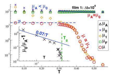
Figure 4-2: Comparison of the different contributions to the shear modulus  $\mu = \mu_{\rm A} - \mu_{\rm F} = (\mu_{\rm A} - \mu_0) + \mu_1$  as functions of T focusing on data obtained for film1 and  $\Delta t = 10^4$ . Inset: Double-logarithmic representation of  $\mu_0/\mu_{\rm A} - 1$  vs T.
