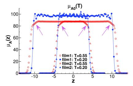
Figure 6-7: Distribution  $\mu_{\rm A}(z)$  of the affine shear modulus  $\mu_{\rm A}$  for film1 and film2 for one temperature in the liquid limit (T=0.55) and one in the glass limit (T=0.20). The midplane plateau  $\mu_{\rm A0}(T)$  is H-independent. As indicated by arrows, surface effects are only strong in the liquid limit.
