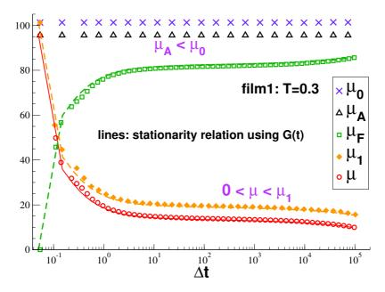
Figure 4-6: Sampling time effects for  $\mu$  and its contributions focusing on film1 and T=0.30. Only the simple averages  $\mu_A$  and  $\mu_0$  are strictly  $\Delta t$ -independent.  $\mu_1$  and (hence)  $\mu$  decrease monotonically. The solid and dashes lines have been obtained using Eq. 1.2.
