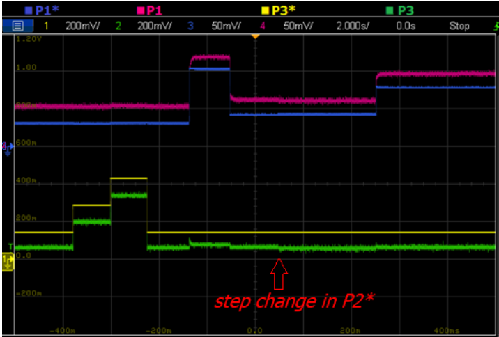
Figure 4.14: Open loop results of a step change in reference powers. The reference values (P1* and p3*) are shown along with their corresponding measured values (P1 and P3).
