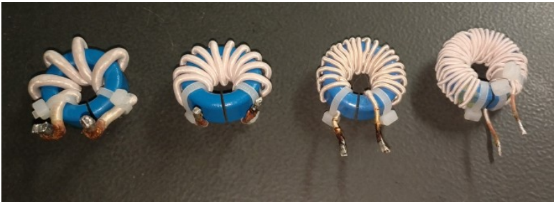
Figure 4.1: The inductors made in G2Elab using a gapped toroid core
