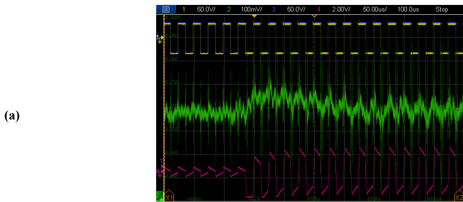
Figure 3.23: Evaluating performance of proposed DC current measurement setup during a power transient. Channels 1 and 3 (yellow and blue) indicate the active bridge voltages of the DAB. Channel 2 (green) is the output of the Hall effect sensor. Channel 4 (pink) is the output of a clamp AC current sensor.
