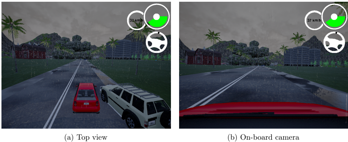
Figure 4.16: Example of a collision with a car invisible from the onboard camera
