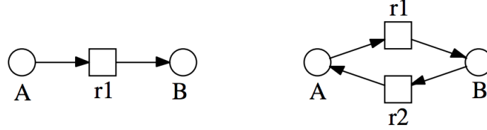
Figure 4.1: Qualitative Petri nets modeling a simple reaction A \rightarrow B (Left) and a reversible reaction A \leftrightarrow B (Right)
