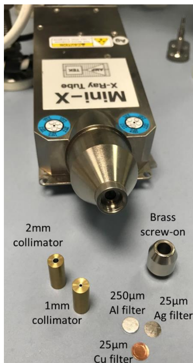
Figure 3.9. Mini X-ray tube with filters and collimators.
