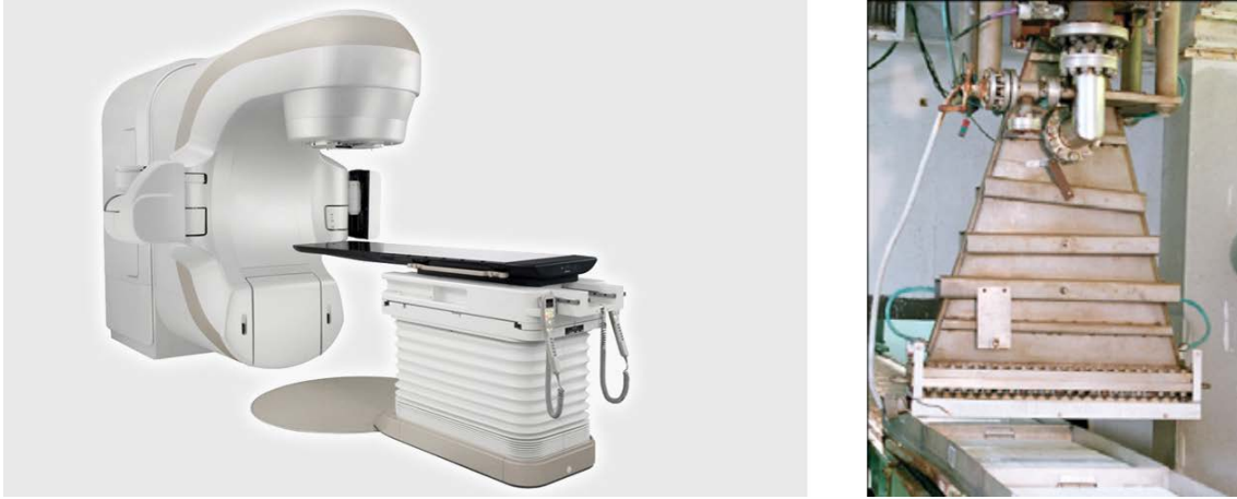
Fig. 1.22 Low-energy electron linac applications. Left: an electron medical linear accelerator (Photo: Varian Medical Systems) [108]; Right: Electron beam technology for sterilising medical products [5]
