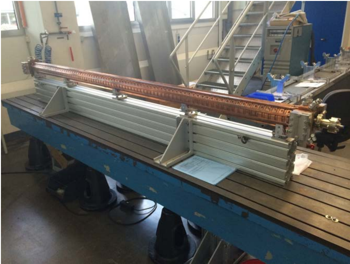
Fig. 3.7 A SLAC-type TW S-band periodic accelerating structure made by RI [95]
