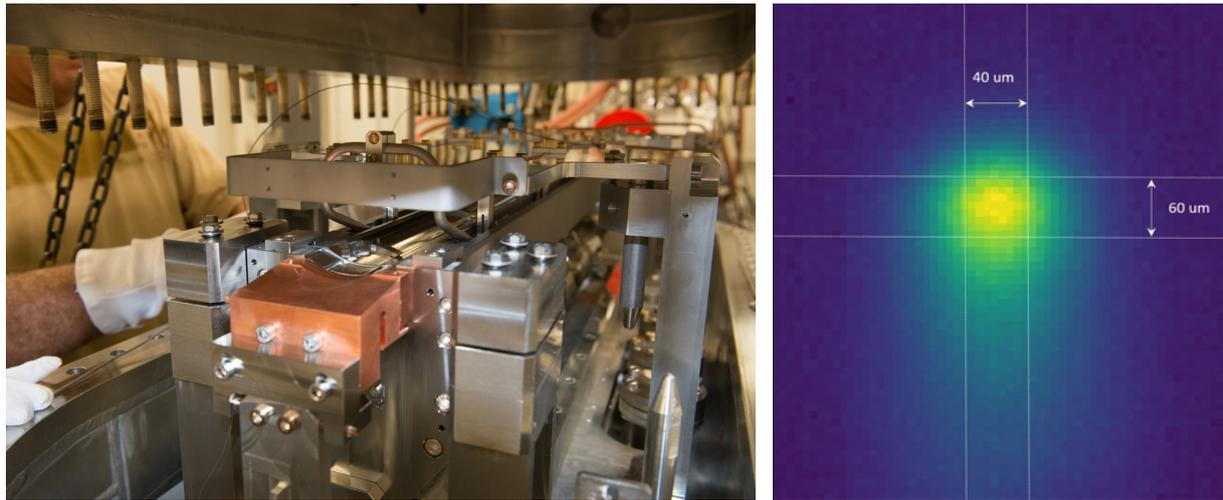
**Figure 3.16:** (a) Thales mirror in the vacuum vessel in the course of installation in EH1. (b) Polychromatic focus on a YAG screen in front of the sample. The beam dimensions are  $40 \times 60 \mu\text{mH} \times \mu\text{mV}$ .
