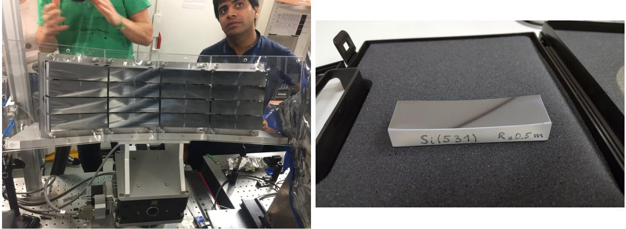
**Figure 3.31:** (a) 16 analysers mounted in the VH holder. When not used, the analysers are protected by a plexiglas screen. (b) Cylindrical Si(531) analyser with a radius of curvature 0.5 m. The analyser is 110 mm wide and 30 mm high. A 0.15 mm crystal wafer is bonded to the glass substrate.
