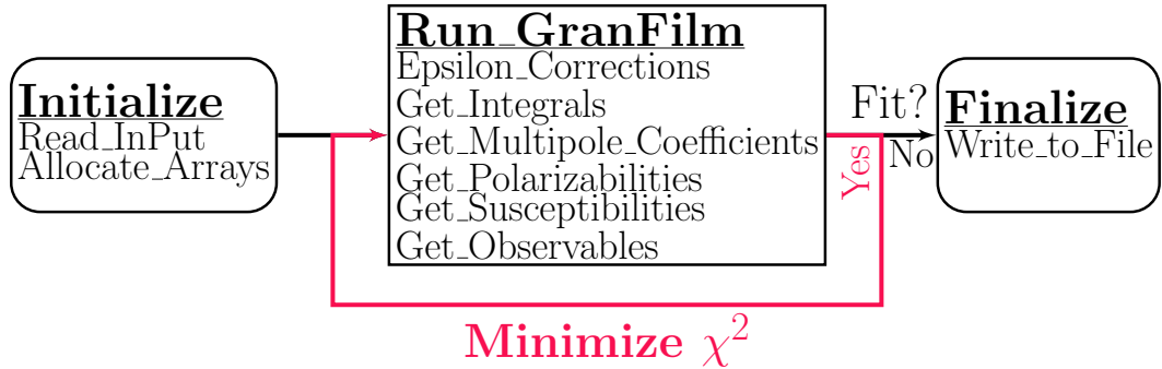
Figure 4.1 A flowchart of the most important steps in a GranFilm simulation. The definition of the system geometry and the allocation of arrays are performed in the initialization process. Next, all the required micro- and macroscopic quantities are calculated in the step Run_GranFilm. The finalization process writes the simulation result to files. If fitting of experimental data is required, the model parameters are adjusted in the step Run_GranFilm until a \chi^2 -minimization criterion is reached.
