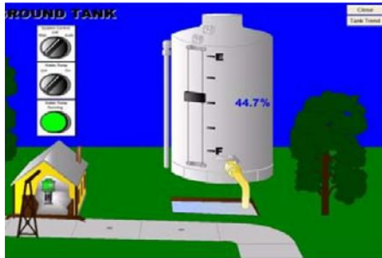
Figure 6.3 – Water Storage Tank HMI Source: [115]
