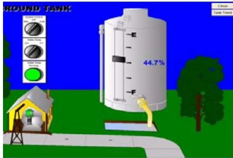
Figure 6.3 – Water Storage Tank HMI Source: [115]
