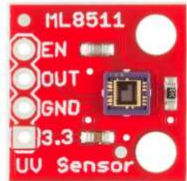
Figure 103: ultra-violet light sensor
