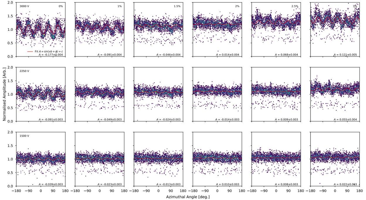
Figure 4.22: Simulated amplitude recorded by an ACHINOS for 5.9 keV photons were generated near the cathode surface and directed within a  $45^\circ$  cone towards the detector centre. Rows correspond to different voltages applied to the Near anodes; columns correspond to successively higher voltages on the Far anode. The distributions were fit with a sinusoidal function, and the amplitude  $A$  is shown for each.
