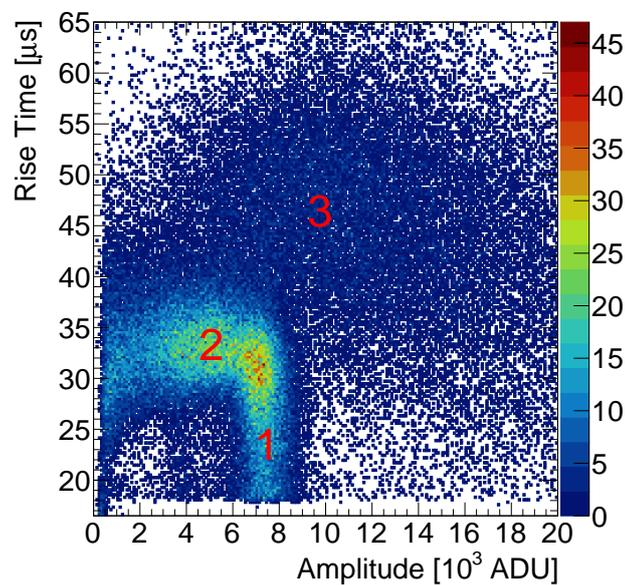
Figure 3.17: Pulse amplitude versus rise time for signals recorded by a 15 cm diameter spherical proportional counter filled with He:Ar:CH<sub>4</sub> (51.7%:46%:2.3%) at 1.3 bar and the 3 mm diameter anode at 2400 V. The labelled population correspond to: (1) 5.9 keV X ray interactions in the gas volume, (2) interactions of the X ray near the cathode surface and (3) cosmic muons. The escape peak is also visible at approximately 4000 ADU.
