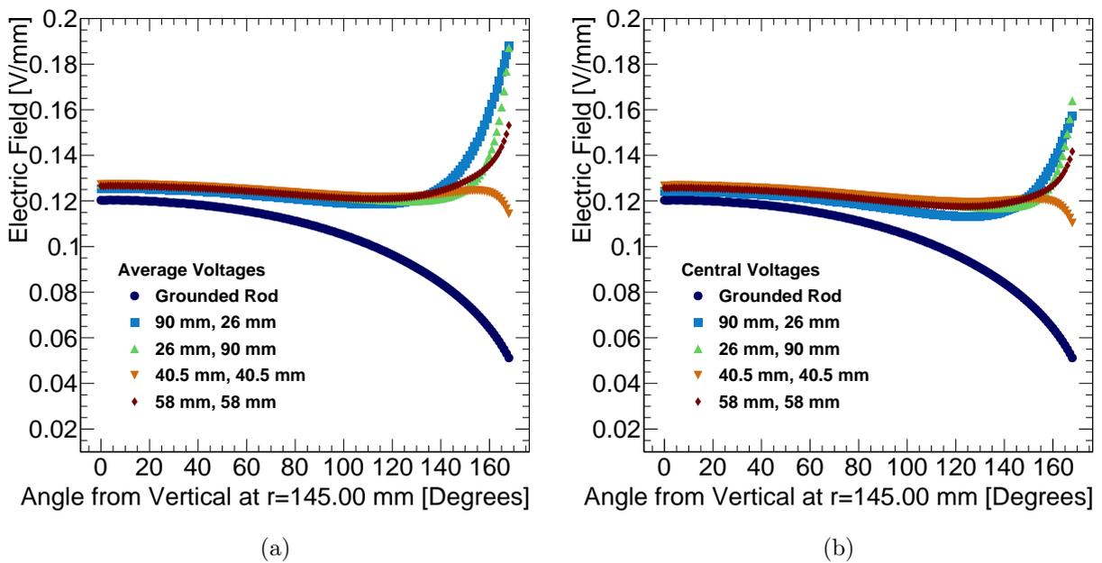
Figure 4.30: Electric field magnitude as function of polar angle at a radius of 145 mm in a  $\varnothing 30$  cm spherical proportional counter for different configurations of segments for the rod in the case where (a) average voltages are applied to the segments and (b) the central voltage is applied to the segment.
