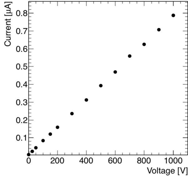
Figure 4.7: Current measured flowing through the glass versus applied voltage. From an average of these measurements, the resistivity of the glass tube was calculated as  $\rho = (5.1 \pm 1.4)10^{10} \Omega \text{ cm}$ .
