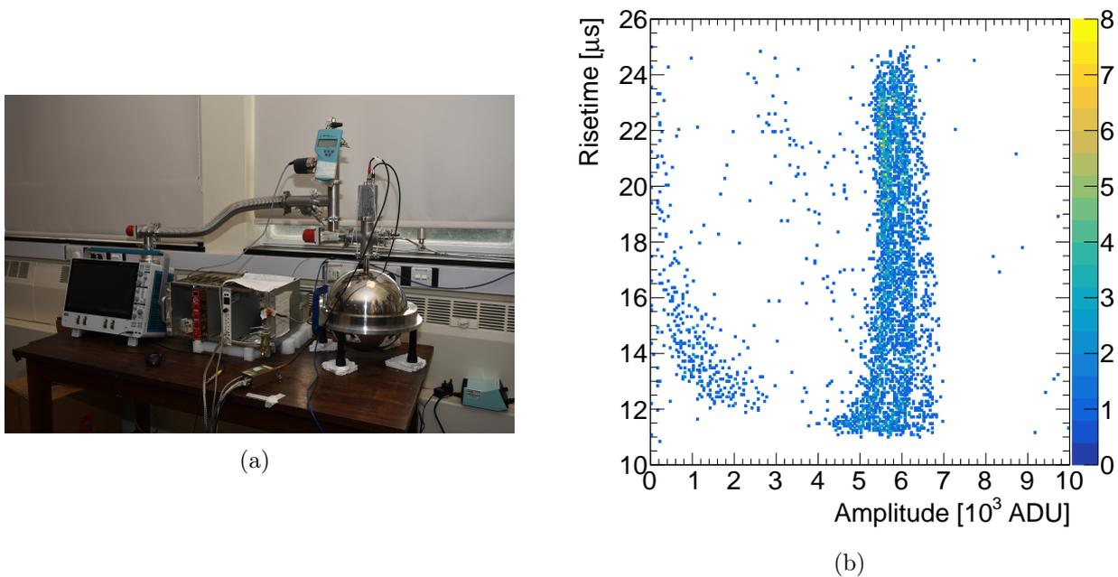
Figure 3.22: (a) A  $\varnothing 30$  cm spherical proportional counter at the University of Birmingham Gaseous Detector Laboratory. Photograph taken by Rhys Owen. (b) Pulse amplitude versus risetime for alpha particles from a triple- $\alpha$  source inside a detector operated with 1 bar N<sub>2</sub>.
