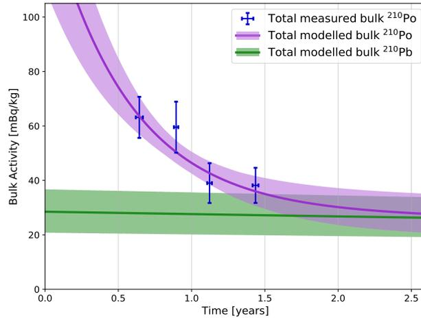
Figure 6.2: Measurements of the  $\alpha$  particles from the decay of  $^{210}\text{Po}$  in a sample of C10100 copper used in the production of the NEWS-G detector. Time is measured from the estimated production date of the copper. The purple (green) line shows the fitted  $^{210}\text{Po}$  ( $^{210}\text{Pb}$ ) activity over time, with the bands showing the  $\pm 1\sigma$  region. Figure reproduced from Ref. [1].
