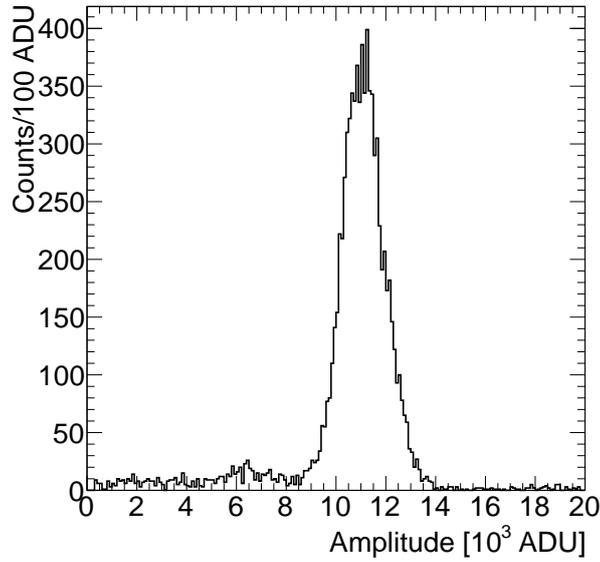
Figure 4.19: Energy spectrum from an  $^{55}\text{Fe}$  source measured using a spherical proportional counter filled with 1000 mbar of Ar : CH<sub>4</sub> (98% : 2%) and using an ACHINOS. The primary peak has an energy resolution ( $\sigma$ ) of  $(7.4 \pm 0.1)\%$ . The second peak, to the left of the main one, is the argon escape peak.
