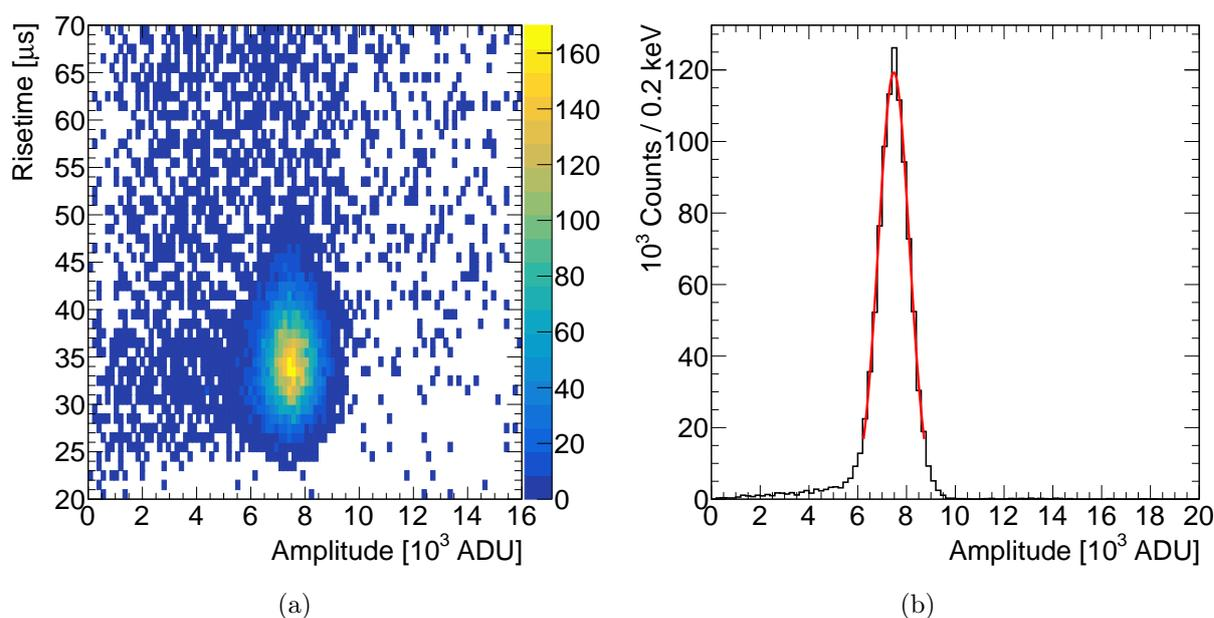
Figure 5.4: (a) Pulse rise time versus amplitude and (b) amplitude distribution for a 6 keV electrons in He:CH<sub>4</sub> (95% : 5%) at 1 bar, after rise time and pulse width selections are applied. The mean of the electron peak is at  $(7.48 \pm 0.01)10^3$  ADU.
