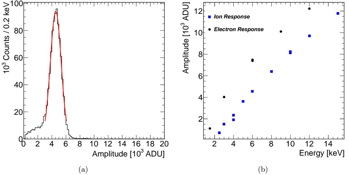
Figure 5.5: (a) Amplitude distribution for 6 keV  $^4\text{He}^+$  ions in He:CH<sub>4</sub> (95% : 5%) at 1 bar with selections applied on the rise time and width to remove cosmic muon background, and fit with a Gaussian distribution. The mean of the peak is at  $(4.55 \pm 0.01)10^3$  ADU. (b) Comparison of the electron and ion amplitudes as a function of particle energy.
