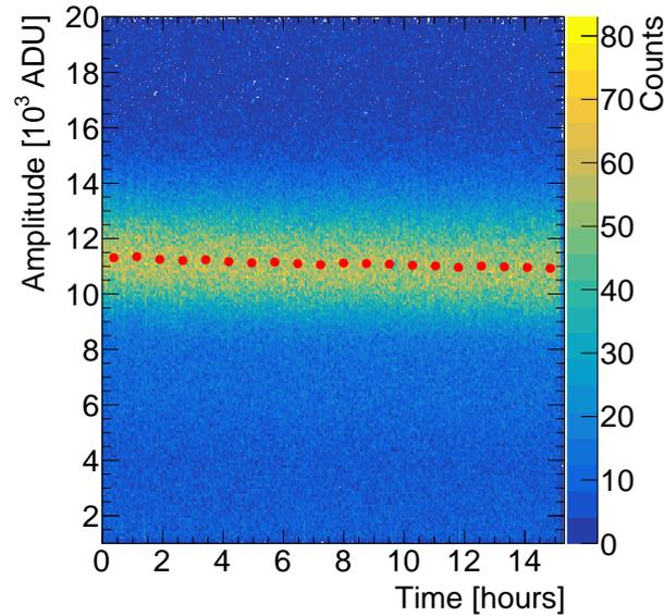
Figure 4.26: Amplitude versus time for a spherical proportional counter filled with 1000 mbar of Ar:CH<sub>4</sub> (98%:2%) and using an ACHINOS. The red points superimposed on the histogram show the mean amplitude in time slices. The slight decrease in amplitude with time is attributed to impurities leaking into the detector.
