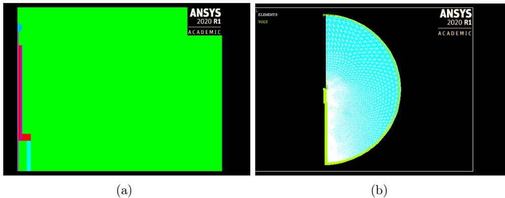
Figure 4.4: Example ANSYS model:(a) close-up of the module in ANSYS and (b) the produced mesh.
