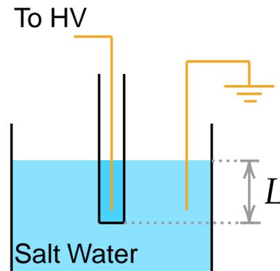
Figure 4.6: Setup of resistivity measurement. The glass tube is filled with and immersed in the solution to depth  $L$ . A voltage is applied across the glass allowing measurement of the current through its volume.
