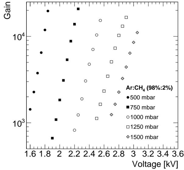
Figure 4.18: Measured amplitude versus the voltage applied to the anode for several pressures of Ar : CH<sub>4</sub> (98% : 2%) in a spherical proportional counter using an ACHINOS.
