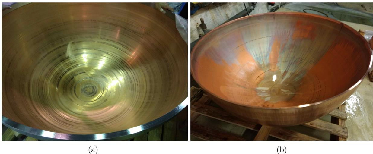
Figure 6.7: A detector hemisphere following (a) initial cleaning with detergent and (b) sanding and chemical etching with an acidified hydrogen peroxide solution. The discolouration observed in the latter is a result of oxidation of the copper and it is removed when the hemisphere is put in contact with the electrolyte.
