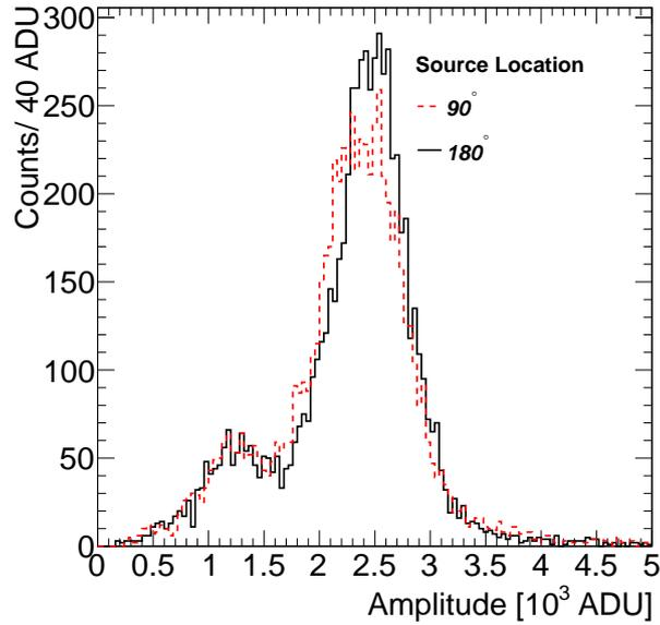
Figure 4.11: The overlaid amplitude distributions for the recorded pulses, for 5.9 keV X rays from an  $^{55}\text{Fe}$  source located inside the detector placed at a zenith angle of  $90^\circ$  (red) and  $180^\circ$  (black), relative to the grounded rod.
