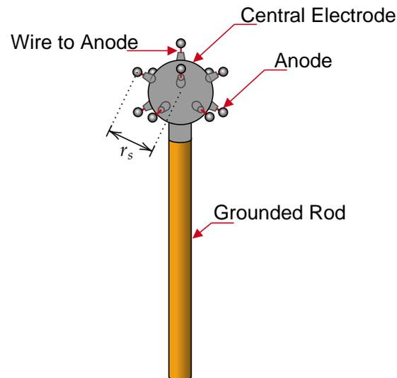
Figure 4.13: Schematic of the multi-anode read-out structure, ACHINOS.
