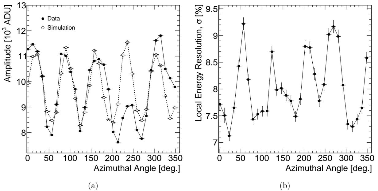
Figure 4.20: Measured and simulated amplitude (a) and measured local energy resolution  $\sigma$  (b) of the 5.9 keV X-ray in a spherical proportional counter with an ACHINOS as a function of azimuthal angle. The detector was operated filled with 1000 mbar of Ar : CH<sub>4</sub> (98% : 2%).
