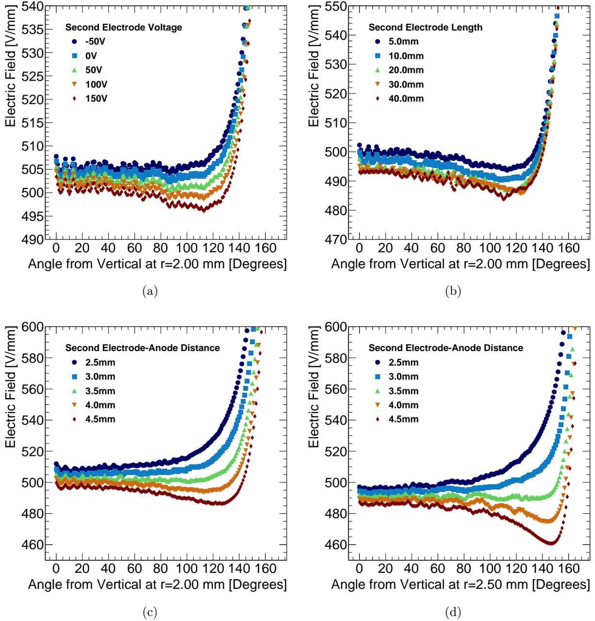
Figure 4.5: Electric field magnitude at 2 mm radius calculated using FEM software for a 15 cm radius spherical proportional counter with a  $\varnothing 2$  mm anode at 2000 V (a), (c) and (b) for varying  $V_2$ ,  $d$  and  $l$ , respectively while the other parameters are fixed at  $V_2 = 200$  V,  $d = 4$  mm and  $l = 5$  mm. (d) shows the electric field magnitude at 2.5 mm in the case of a  $\varnothing 3$  mm anode for various values of  $d$ , keeping all other parameters the same as (c).
