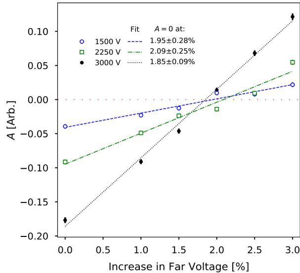
Figure 4.23: Amplitude  $A$  of sinusoidal function from fits in Fig. 4.22 as a function of the percentage increase in voltage applied to the Far anodes for three voltages applied to the Near anodes. A linear fit was applied to each data set and the increase in Far voltage required for  $A = 0$  (red dotted line), which is considered to have the most homogeneous field, is given.
