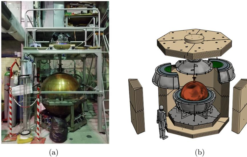
Figure 3.20: (a)  $\varnothing 140$  cm spherical proportional counter, SNOGLOBE, during the commissioning phase in LSM and (b) its shielding of 3 cm archaeological lead, 22 cm low radioactivity lead and 40 cm high-density polyethylene (HDPE), reproduced from Ref. [1].
