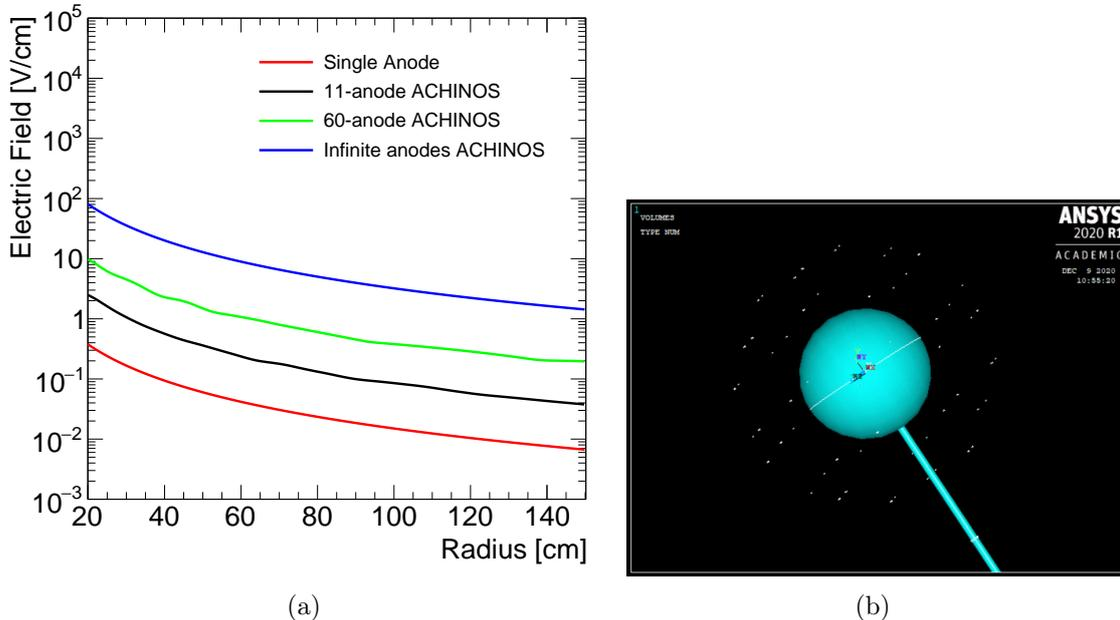
Figure 4.28: (a) Electric field magnitude as a function of radius for a  $\varnothing 3 \text{ m}$  spherical proportional counter for various read-out modules, each using  $\varnothing 1 \text{ mm}$  anodes and an ACHINOS radius  $r_s$  (distance between each anode and the centre) of 10 cm. ‘Infinite anodes ACHINOS’ refers to the approximation where there are an infinite number of anodes all located at  $r_s$ . (b) The ANSYS model of the prototype 60-anode ACHINOS.
