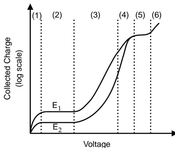
Figure 3.11: Modes of detector operation for gaseous detectors. The collected charge is plotted as a function of voltage for two different energies deposited in the gas ( $E_1 > E_2$ ). The labels regions are: (1) recombination before total charge collection; (2) ionisation mode; (3) proportional mode; (4) region of limited proportionality; (4) Geiger-Müller mode; (5) discharge region.
