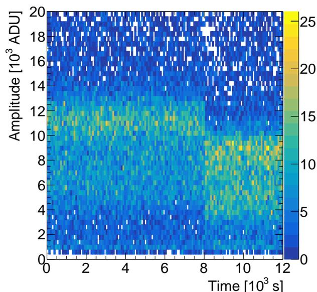
Figure 4.10: Amplitude versus time in a module with a second correction electrode. Initially, the second correction electrode voltage was at 100 V but was increased to 200 V at 8000 s.
