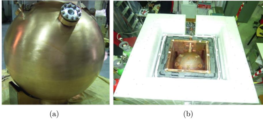
Figure 3.18: (a)  $\varnothing 60$  cm spherical proportional counter, SEDINE, and (b) shielding of 8 cm copper, 15 cm lead and 30 cm polyethylene. Figures reproduced from Ref. [144] and Ref. [135], respectively.
