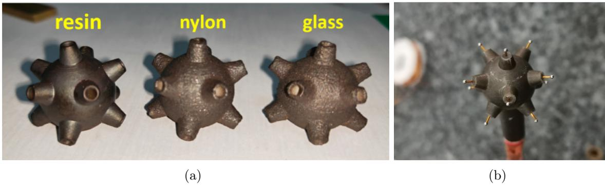
Figure 4.16: (a) Three different support materials (resin, nylon, glass) covered with a DLC layer. Figure reproduced from Ref. [4]. (b) An 11-anode ACHINOS constructed using a DLC-coated support structure.
