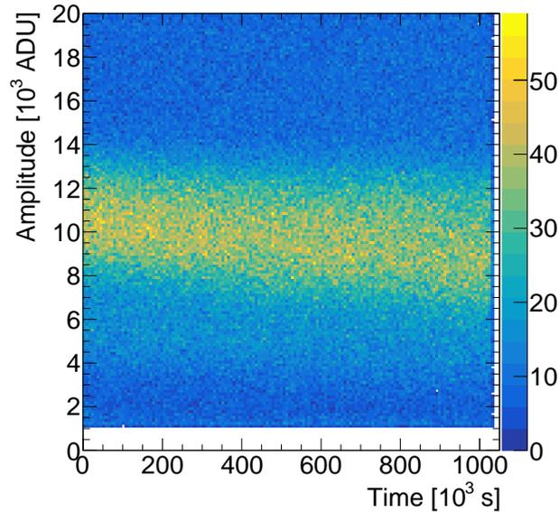
Figure 4.12: Pulse height as a function of time recorded using a module with a second correction electrode at 0 V, with an anode voltage of 2350 V in a detector filled with 2 bar of He:Ar:CH<sub>4</sub> (87%:10%:3%). The decrease in pulse height over time is due to contaminants, such as oxygen, leaking into the detector. Detector operation is stable and no discharges are observed.
