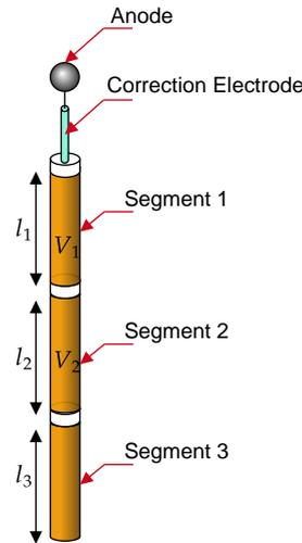
Figure 4.29: Schematic of the segmented rod correction electrode.
