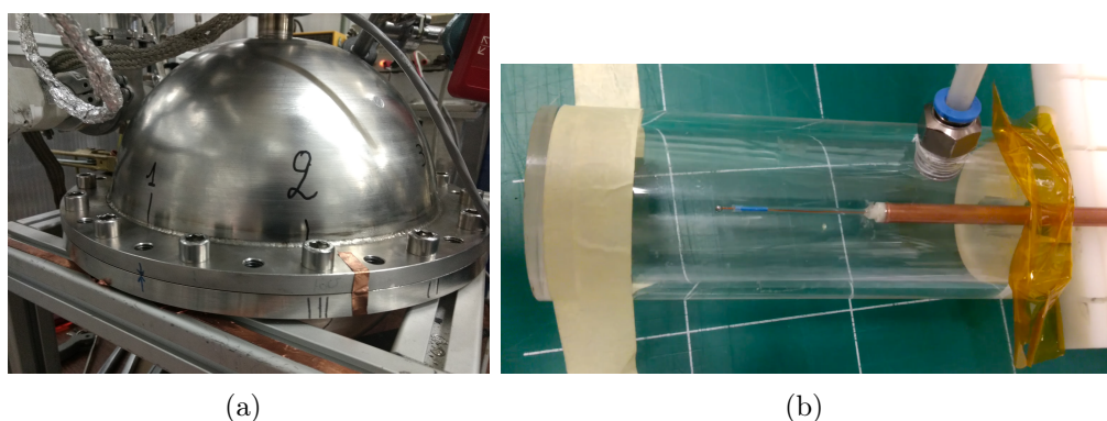
Figure 4.9: (a) \varnothing 30 cm stainless steel spherical proportional counter used for tests in CEA Saclay. (b) the chamber used for testing modules for sparks.
