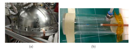
Figure 4.9: (a)  $\emptyset$  30 cm stainless steel spherical proportional counter used for tests in CEA Saclay. (b) the chamber used for testing modules for sparks.
