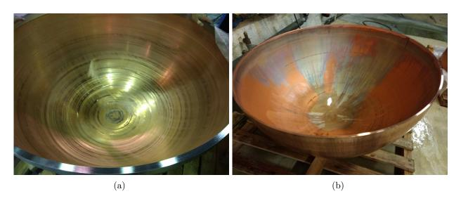
Figure 6.7: A detector hemisphere following (a) initial cleaning with detergent and (b) sanding and chemical etching with an acidified hydrogen peroxide solution. The discolouration observed in the latter is a result of oxidisation of the copper and it is removed when the hemisphere is put in contact with the electrolyte.
