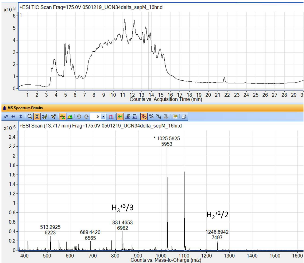
Figure S3. LC-MS of UCN34 \Delta sepM supernatant after 16 hours incubation. Sgg GSP expected: H_2^{+2}/2 [1246.6855 Da] and H_3^{+3}/3 [831.4594 Da].
