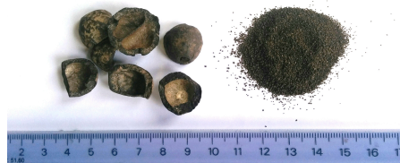
Figure 2.1: Coconut endocarp (on the left) and grinded fine particles of coconut endocarp (on the right).
