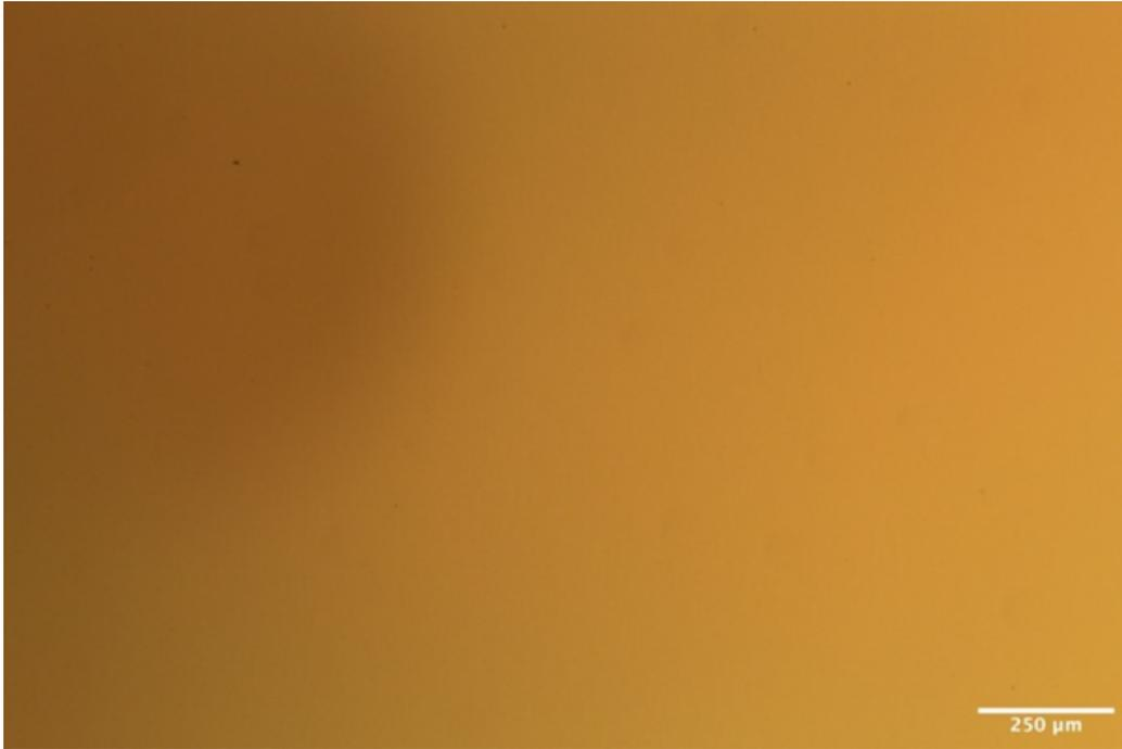
Figure 4.3: Optical microscope image of an adhesive-bonded Si-Si sample showing a bubble-free interface.
