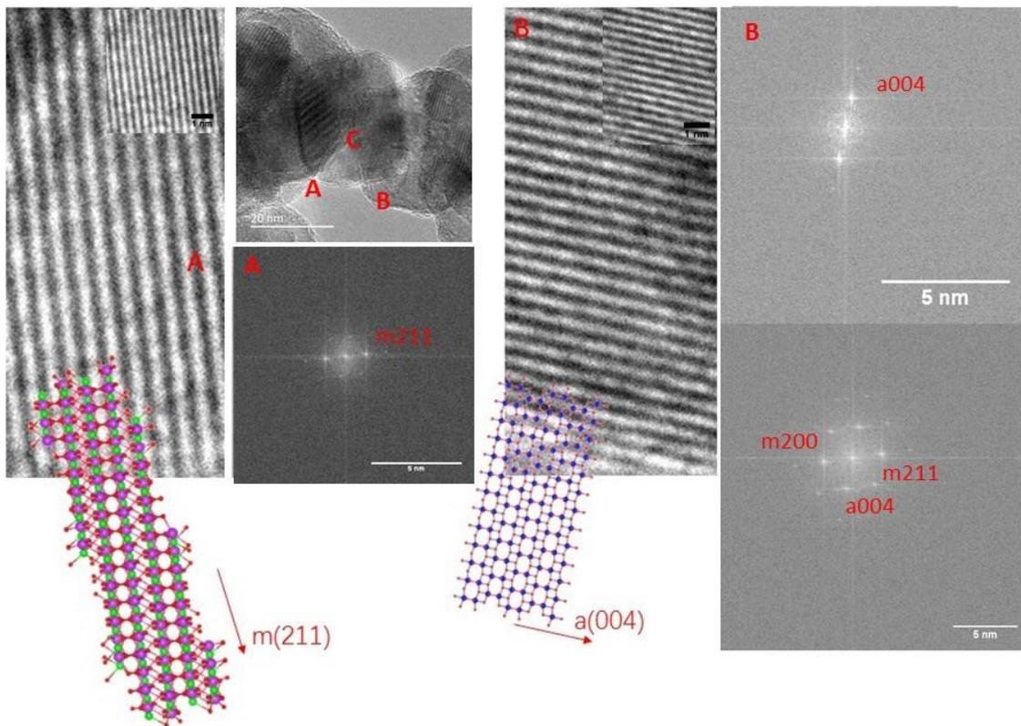
**Fig. 3.8** TEM micrograph, FFT planes, and simulated crystalline models for the 0.8:0.2 composite. Regions A, B, and C correspond to pure BVO, TO, and the junction of both crystalline phases, respectively.
