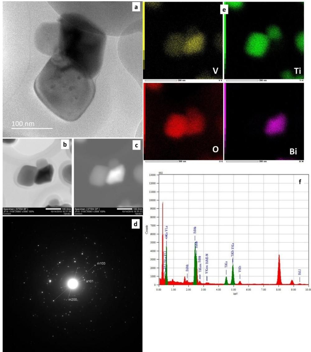
**Fig. 3.7C** Micrograph of the nanocomposite 0.2:0.8 a) isolated particles b) bright-field image c) dark field image d) FFT diffraction pattern e) elemental mapping of the nanocomposite f) EDS analysis of the nanocomposite.
