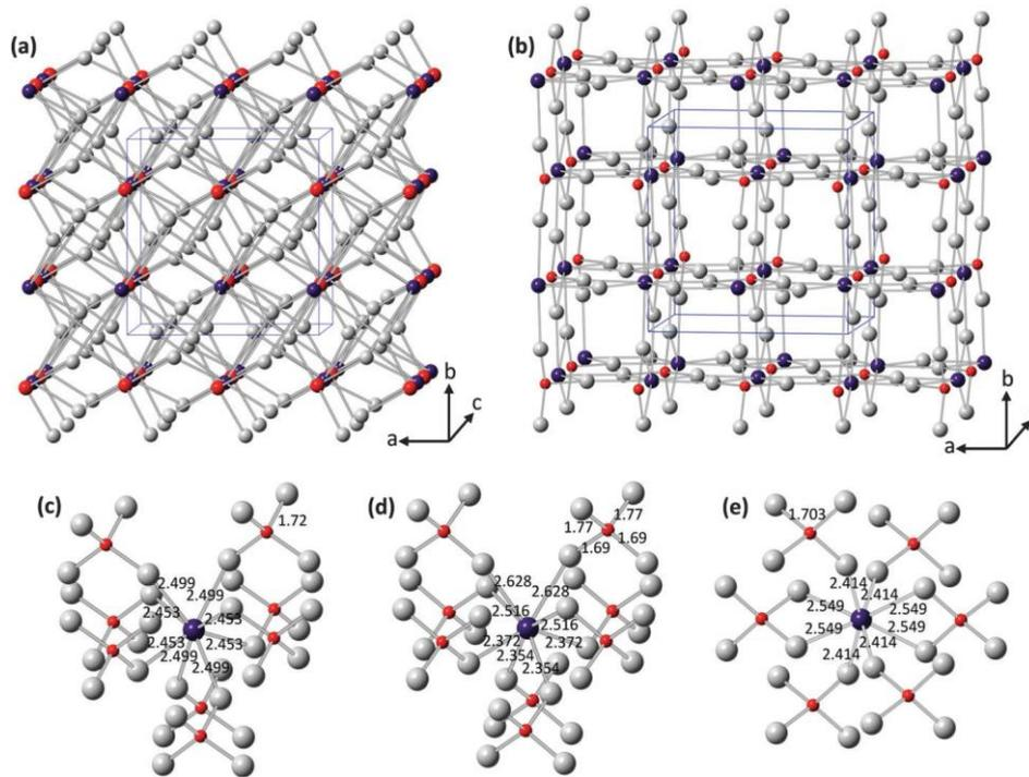
**Fig. 1.8** (a) Tetragonal- scheelite structure (b) Tetragonal- zircon structure [ red; vanadium, purple; bismuth, grey; oxygen]. The monoclinic- scheelite structure is similar to tetragonal scheelite as in (a) except for changes in atomic positions of Bi, V, and O atoms [47]
