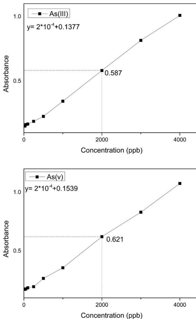
**Fig. 4.7** Calibration curves for As(III) and As(V)
