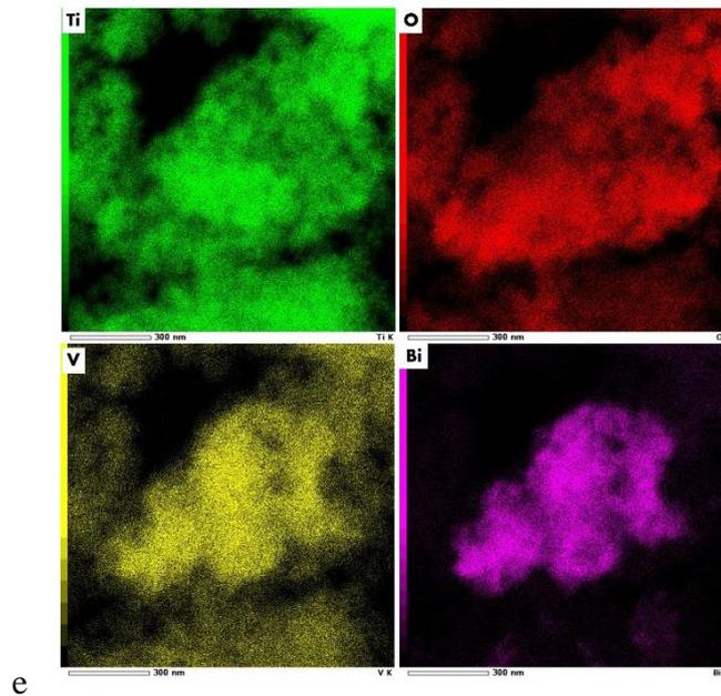
**Fig. 3.7A** Micrographs of the 0.8:0.2 nanocomposite a) TEM micrograph of the whole area b) Selected area from the sample c) FFT diffraction pattern d) EDS chemical analysis e) Mapping of the samples.
