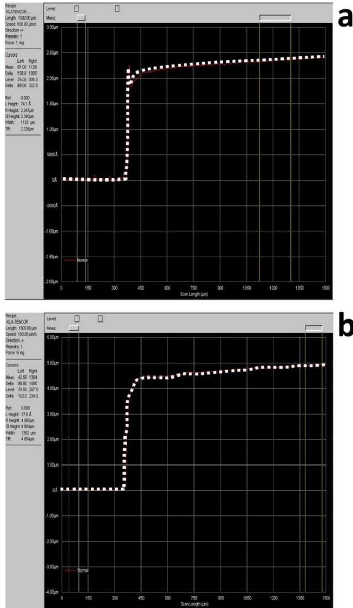
**Fig. 5.15** a) Thickness measurement for the layered film b) Thickness measurement for the nanocomposite film
