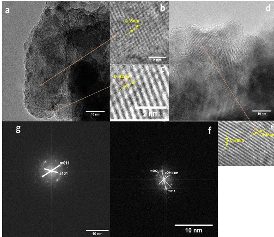
**Fig. 5.12** TEM Micrograph of the films deposited over Ceramic substrates a) Layered film b,c) Cropped planes d) Composite ceramic film e) Cropped planes from the composite film f,g) FFT from the layered and composite films respectively
