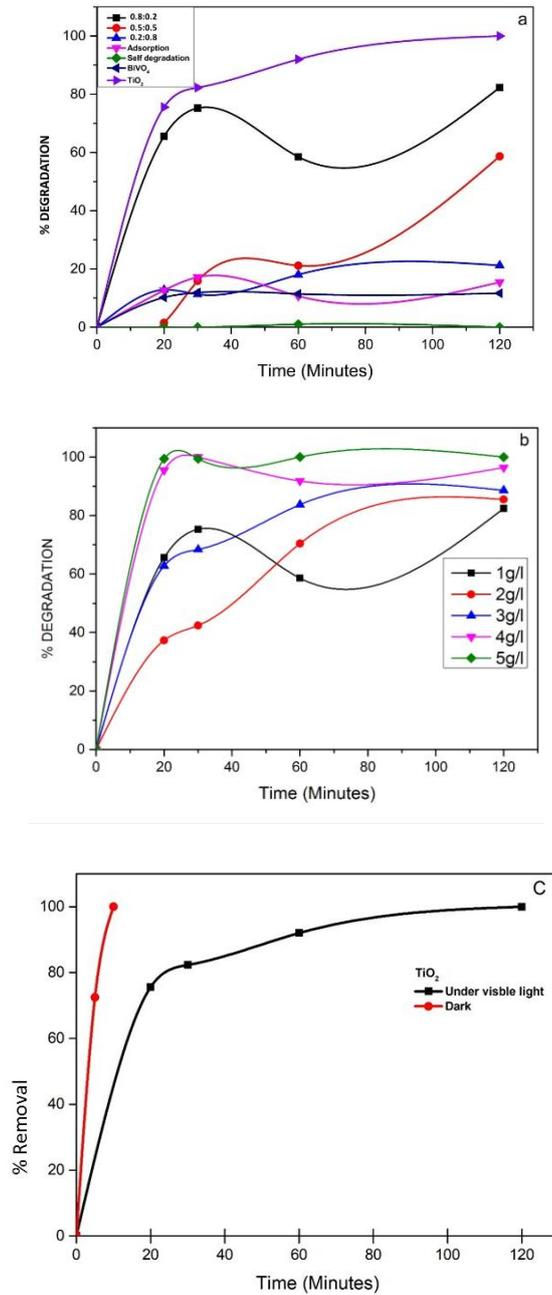
**Fig. 3.9** Pc degradation of AB113 measured for wavelength of 568 nm (a) Adsorption and self-degradation plots along with the comparison of pc activity of TO, BVO and the three nanocomposite ratios  $[\text{AB113}]_0 = 40$  mg/l,  $[\text{nanocomposite, TO, BVO}] = 1\text{g/l}$   $\text{pH}_0 = 6$ . (b)  $[\text{AB113}]_0 = 40$  mg/l,  $[\text{nanocomposite}] = 1\text{-}5\text{g/l}$   $\text{pH}_0 = 6$  (c) Comparison of the activity of TO (Both adsorption and photocatalysis)
