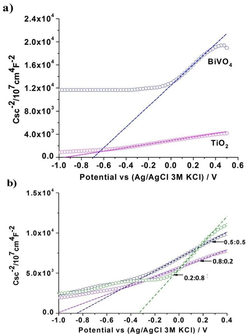
**Fig. 3.11** Mott-Schottky curves of (a) BVO and TO and (b) TO/ BVO nanocomposites (0.8:0.2, 0.5:0.5, and 0.2:0.8) compositional ratio BVO: TO). The  $C_{sc}$  were obtained at 100 Hz in 0.05 M NaClO<sub>4</sub> aqueous solution.
