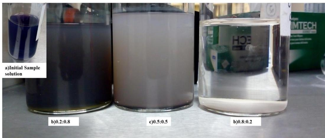
**Fig. 3.10** The preliminary AB113 degradation test by each sample [Dosage] = 1g/l [C<sub>0</sub>] = 40mg/l The reaction constant was determined from the corresponding kinetic plot from the reaction, which follows pseudo-first-order kinetics [15].
