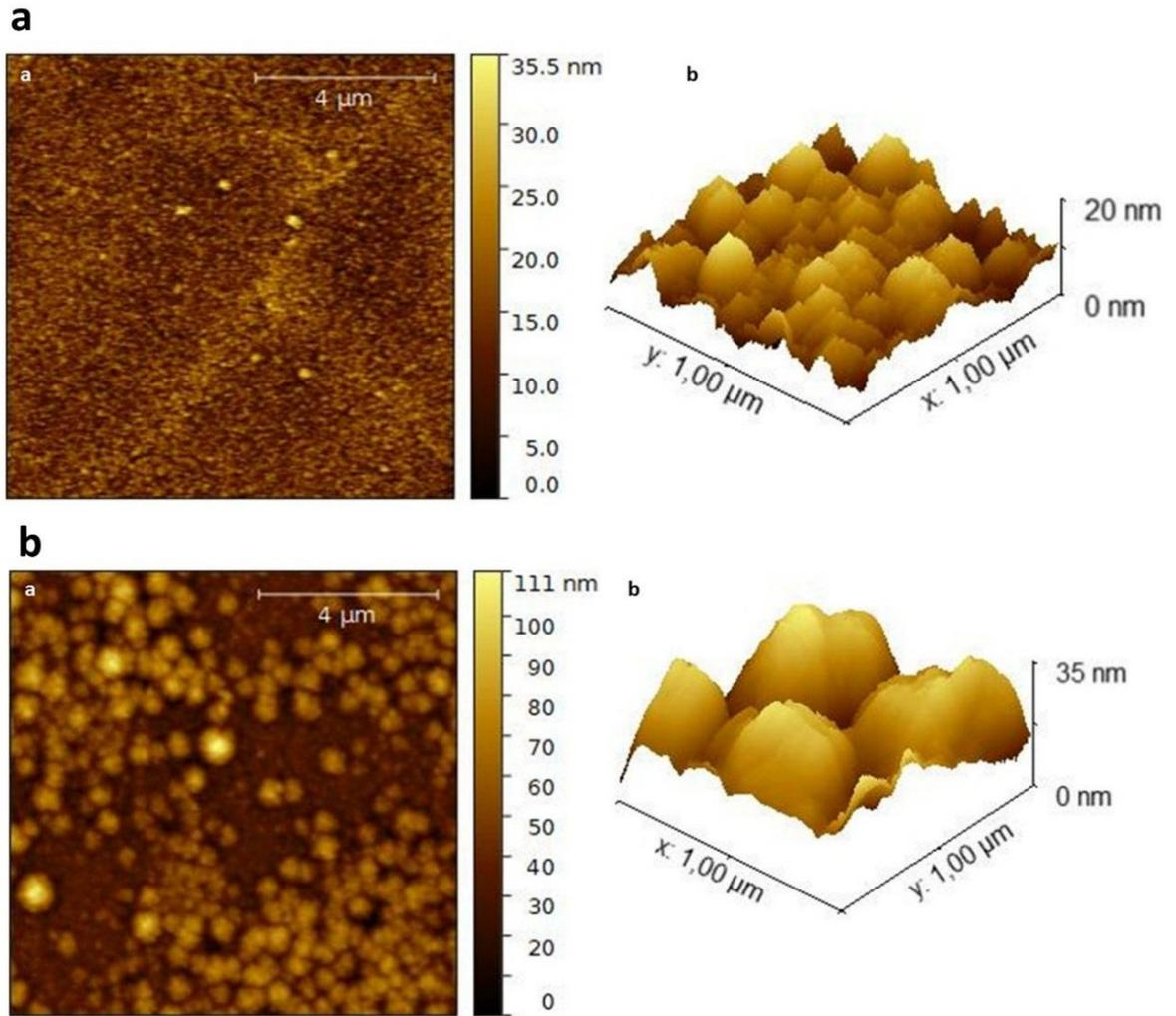
**Fig. 5.16** a) Morphology of the layered film deposited on BK7 substrate by AFM- both a) 2D and b) 3D images, respectively, are illustrated b) Morphology of the composite film deposited on BK7 substrate by AFM- both a) 2D and b) 3D images, respectively
