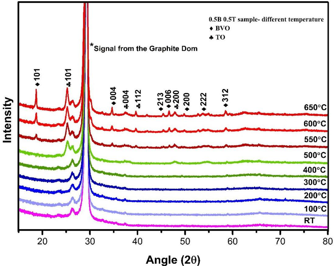
Fig. 5.4 In-situ annealing X-ray diagrams of the nanocomposite film (Optimization of the annealing temperature)
