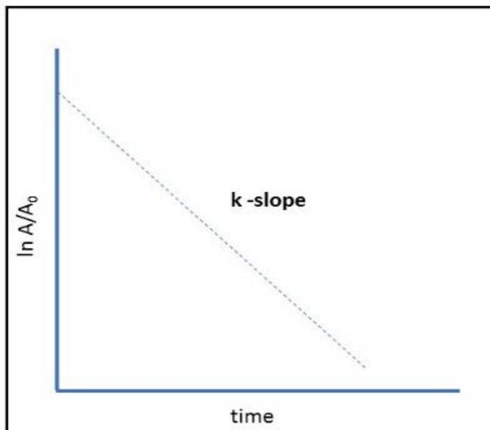
**Fig.2.20** Plot of the reactant concentration versus time for a first-order process
