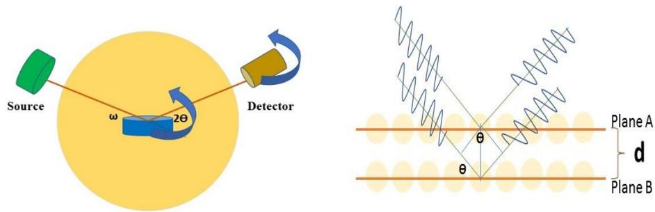
**Fig. 2.5** Illustration of the principle of xrd.
