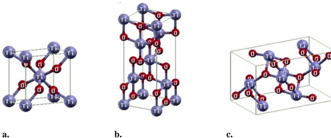
**Fig. 1.6** a) Rutile b) Anatase and c) Brookite phases of TO [38]
