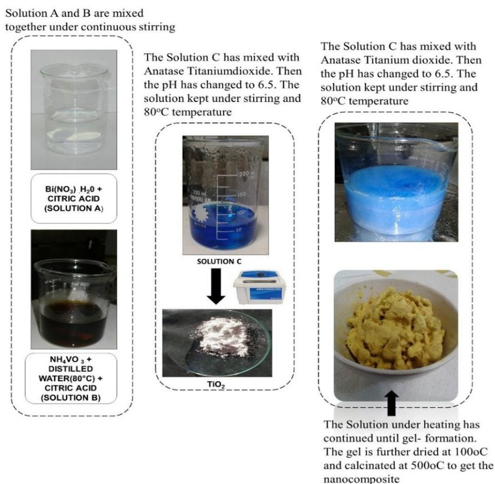
**Fig. 2.1** Sol-gel Synthesis step
