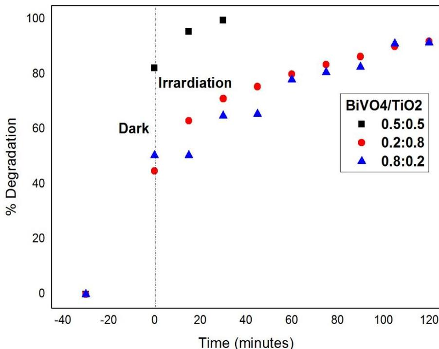
Fig. 5.17 Pc test for choosing the best composite; Methylene blue
