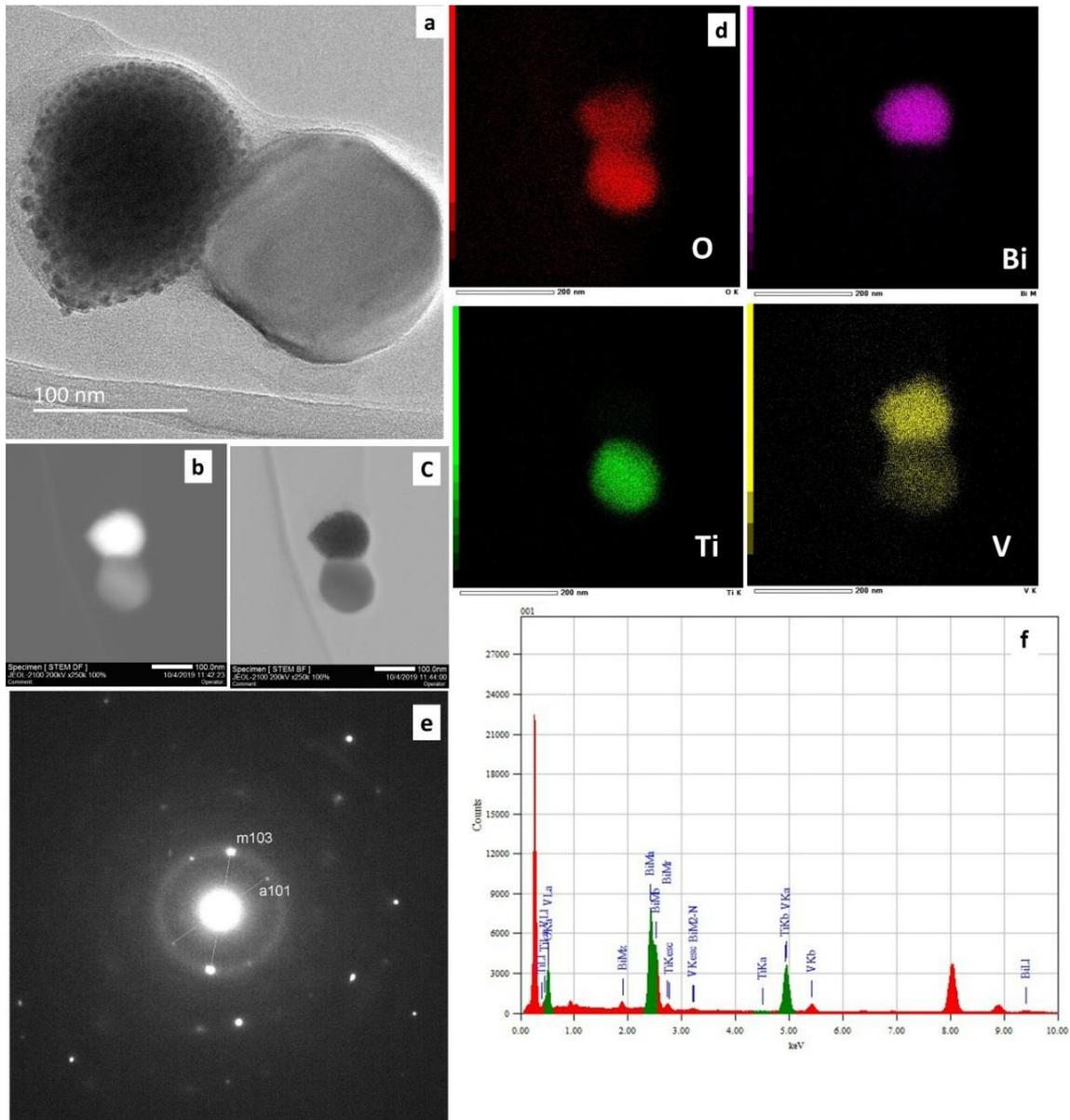
**Fig. 3.7B** Micrographs of the 0.5:0.5 nanocomposite a) TEM micrograph of isolated particles b,c) bright and dark field analysis d) Mapping analysis of sample e) FFT diffraction pattern f) elemental mapping and f)EDS analysis, respectively
