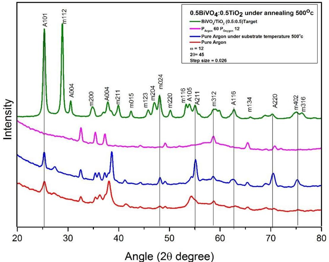
**Fig. 5.2** X-ray diagrams of the composite film deposited under different chamber atmosphere
