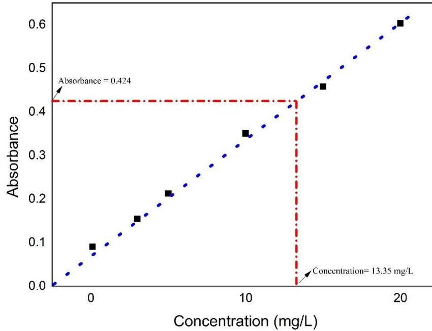
**Fig. 2.19** Calibration curve- Absorbance Vs. Concentration
