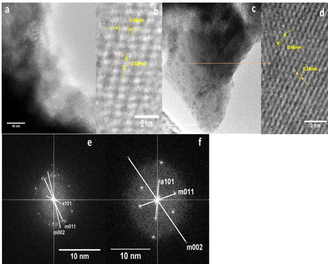
**Fig. 5.11** TEM Micrograph of the films deposited over BK7 substrates a) Layered film b) Planes from the layered film c) Composite film d) Cropped planes from composite film e,f) FFT of the layered and composite films respectively
