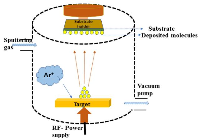
Fig. 2.3 Schematic representation of the sputtering process
