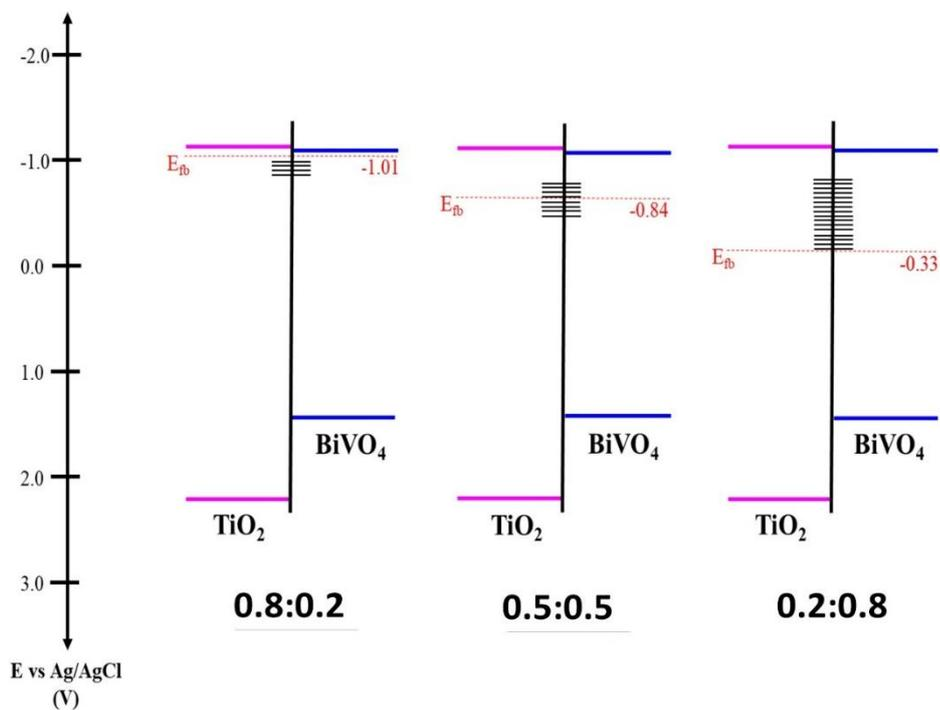
**Fig. 3.12** Energy diagram proposed for TO/ BVO nanocomposites (0.8:0.2, 0.5:0.5 and 0.2:0.8 compositional ratio)
