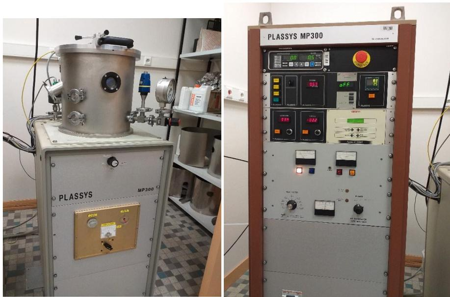
Fig. 2.2 Plassys MP300 RF sputtering equipment
