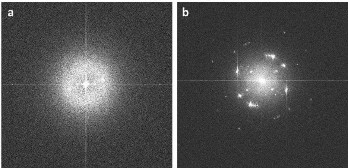
**Fig. 2.13** FFT of a) amorphous and b) crystalline samples.
