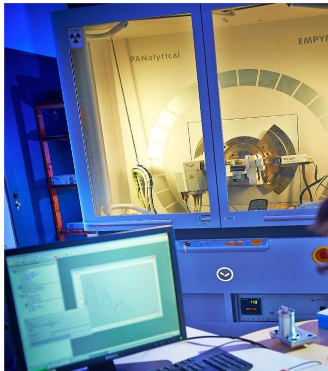
**Fig. 2.6** PANalytical Empyrean X-ray diffractometer
