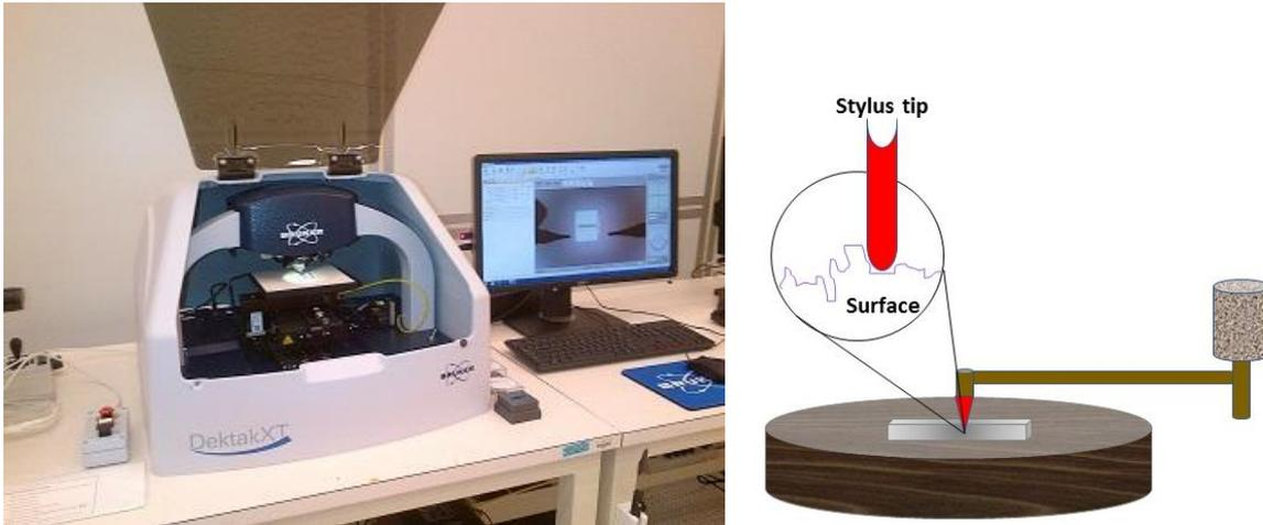
**Fig. 2.15** Dektak XT profilometer- with schematic diagram
