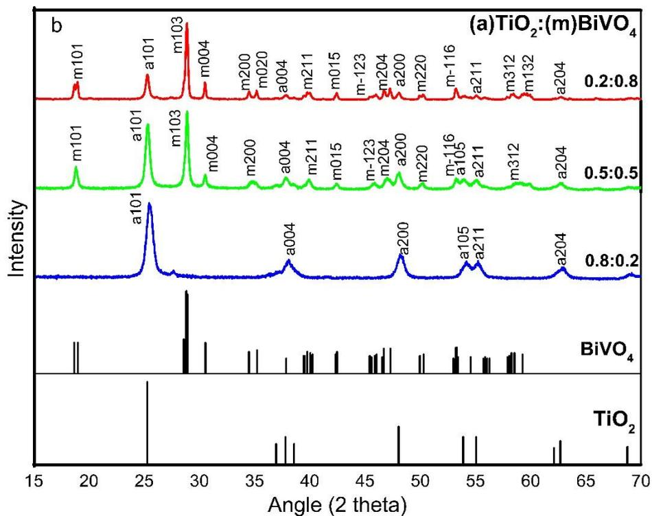
**Fig. 3.3** Xrd patterns of the nanocomposites a) before and b) after calcination (500°C), compared with those of pure TO (JCPDS 00-021-1272) and sol-gel synthesized BVO (JCPDS-00-075-1866). Before the
