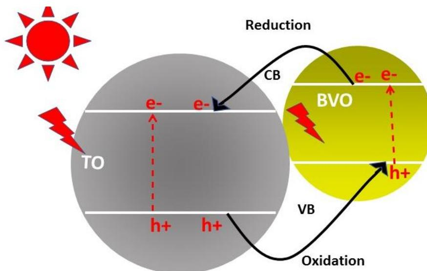
**Fig. 1.5** Photocatalysis scheme for coupled semiconductors system
