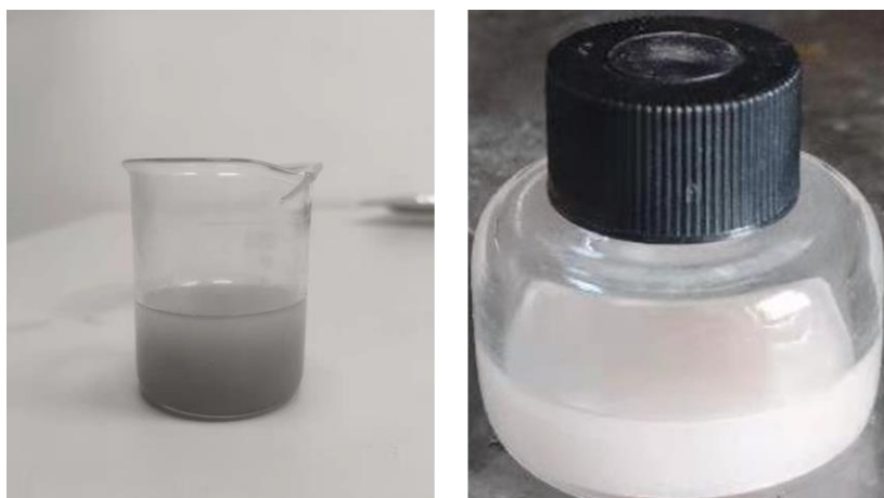
Figure 7.7 Color change of solution before (left) and after (right) catalysis with MAPbI 3 /TiO 2 as catalyst
