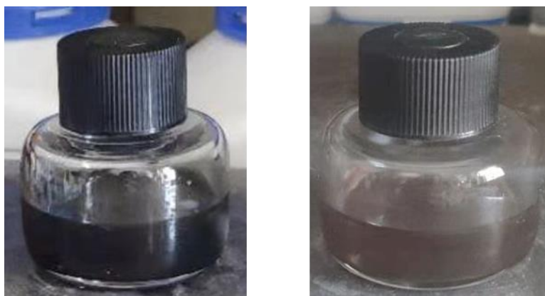
Figure 7.6 Color change of solution before (left) and after (right) catalysis with MAPbI 3 as catalyst
