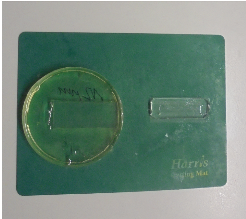
FIGURE 2.3: Photography of a wafer containing the PDMS and curing agent mixture (left) and the final microfluidic chip after bonding it to a glass slide with plasma exposure (right)
