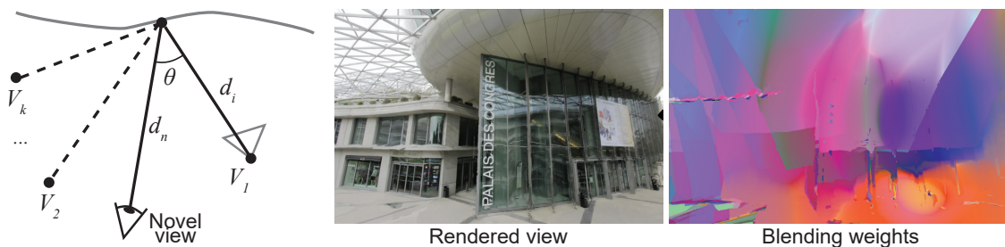
Figure 2.12 – The ULR blending weights at a point on the surface take into account the distances from that point to the input view d_i and novel view d_n , along with their relative incidence angle \theta and the location in the input image space. The best cameras are ranked and their scores normalized.
