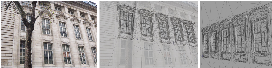
Figure 3.11 – For each platonic camera, we estimate the transformation to align it back to the corresponding estimated camera in the input scene. We use this transformation to copy the platonic mesh at each window occurrence in the facade.
