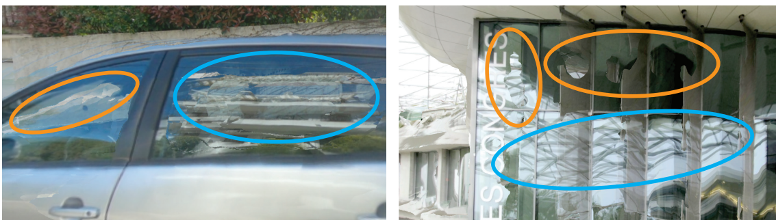
Figure 1.6 – Artifacts introduced by reflective and transparent surfaces: missing or erroneous geometry caused by specularly or transparency (orange), duplicated or blurry reflections caused by an erroneous flow (blue).
