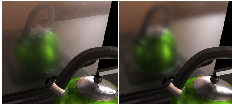
Figure 5.15 – Left: glossy layered rendered by gathering from probes generated using initial material roughness. The reflections are sharper. Right: our glossiness convolution applied on halved roughness probes approximate the effect of the material full roughness.
