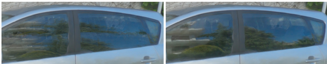
Figure B.2 – A comparison between a planar (left) and ellipsoid (right) representation for each window when computing the reflection flow. The planar simplification leads to strong alignment artifacts and duplications.
