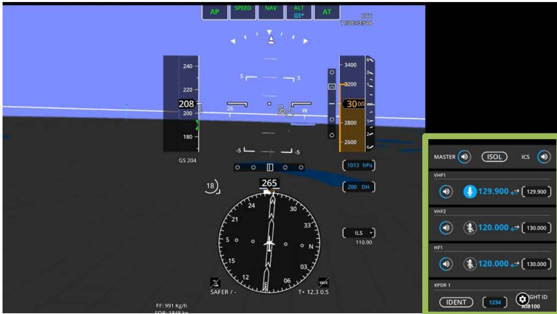
**FIGURE 48 – VUE DU PFD AVEC CARTOUCHE VHF DANS LA PARTIE DROITE
