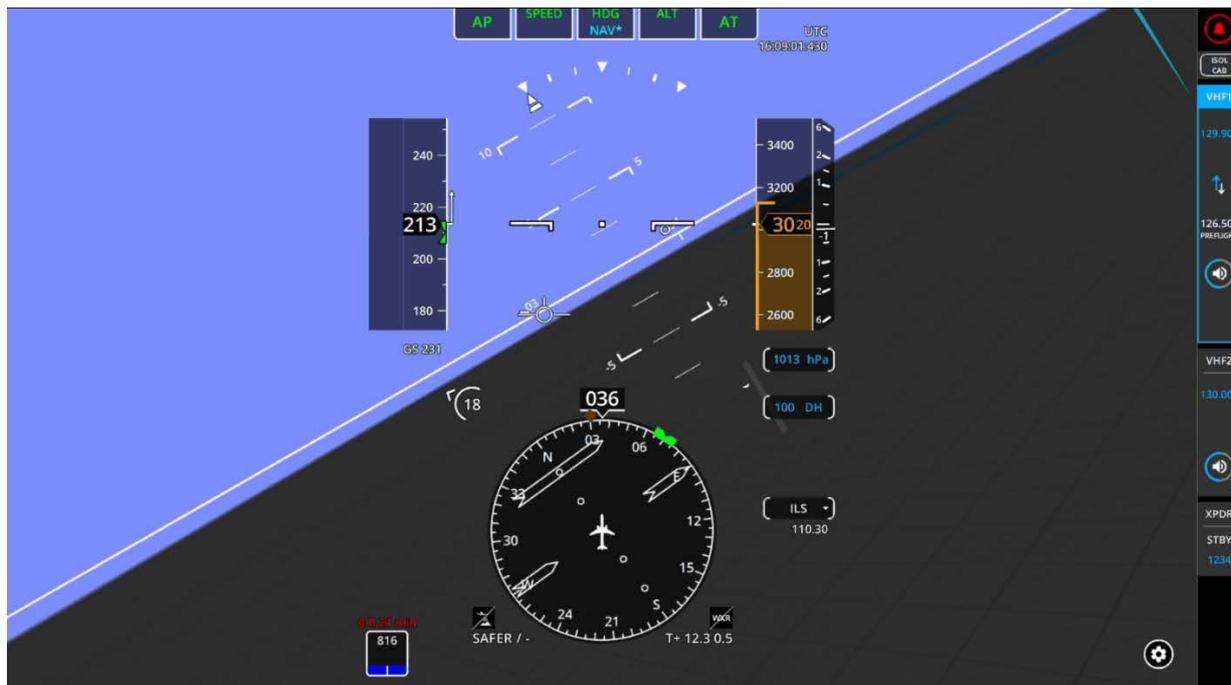
**FIGURE 59 – VUE DU PFD AVEC UN TEMPS DE VOL RESTANT <30MIN (D'APRÈS CARBURANT)**
