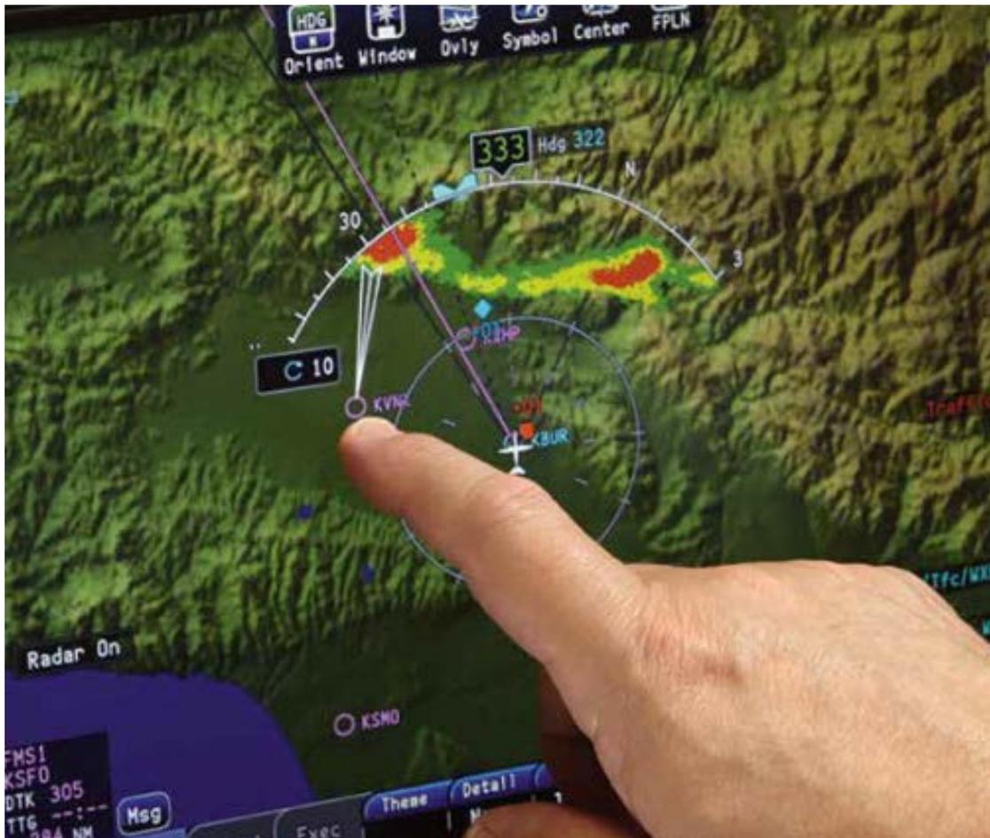
**FIGURE 37 – INTERFACE DE ROCKWELL-COLLINS AVEC UNE INTERACTION DIRECTE AVEC LA CARTOGRAPHIE.**
