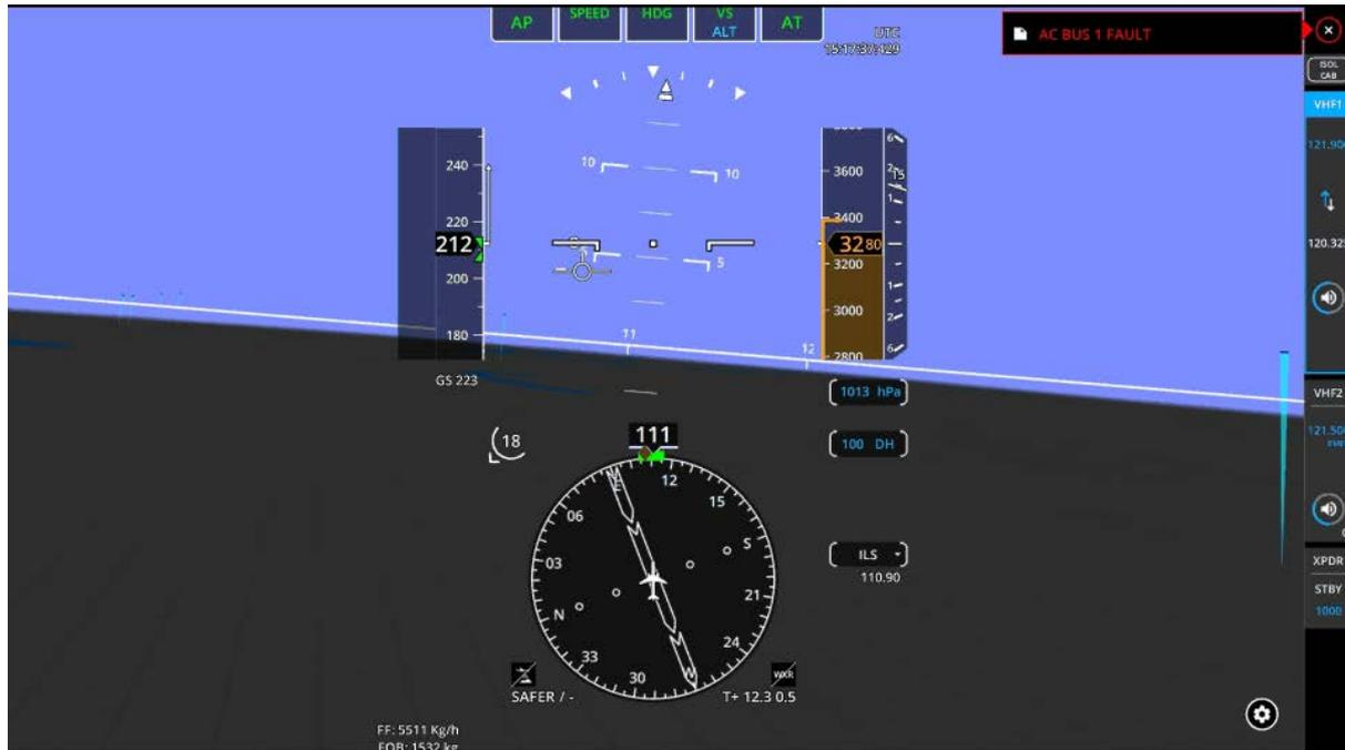
**FIGURE 51 – VUE DU PFD AVEC LE BOUTON D’OUVRIR LA PROCÉDURE ECAM EN HAUT À DROITE**
