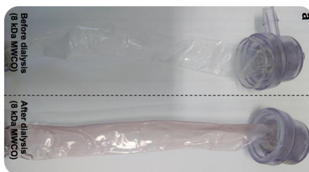
Fig. 92 Dialysis of PF at 8kDa molecular weight cut-off.
