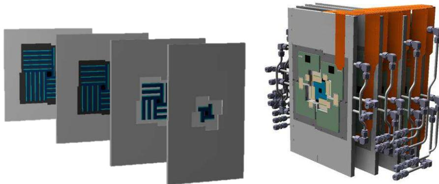
*Figure 1.4 The geometry of MVD for CBM.*
