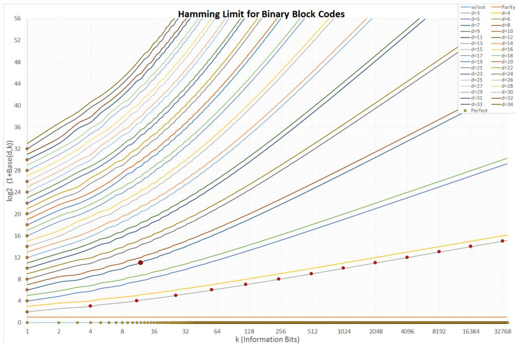
Fig. 3.4. The hamming limit of binary block codes [4].
