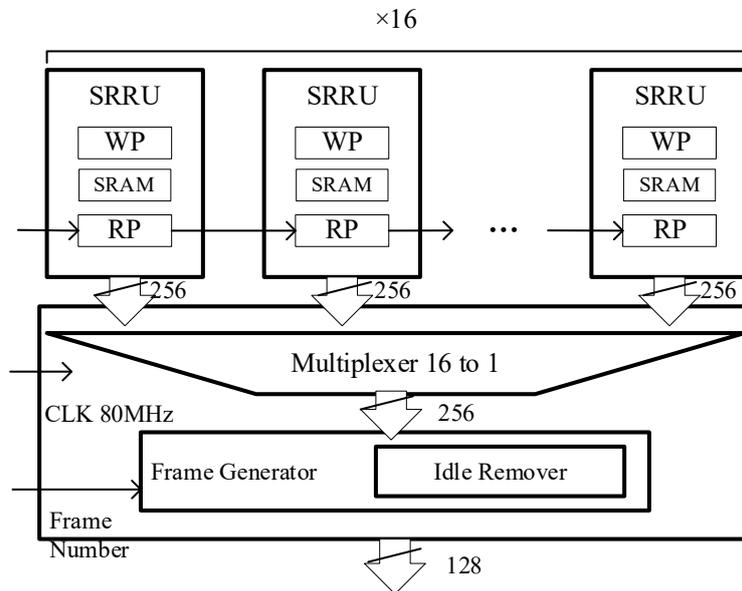
Figure 4.5. The block diagram of the Multiplexer and Frame Generator.
