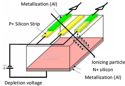
Figure 1.8 The principal of the silicon strip detector.
