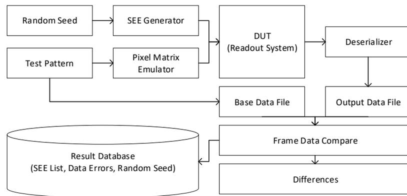
Figure 4.23. The evaluation data path of the readout system.
