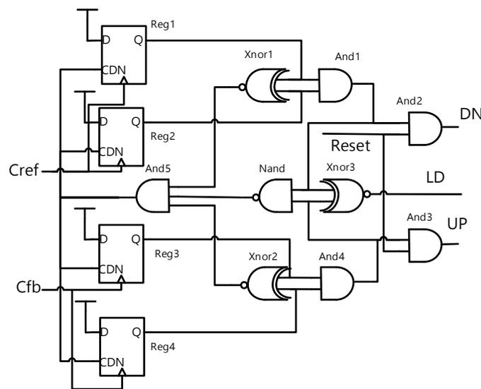
Figure 5.15. The schematic of PFD with DMR implemented.
