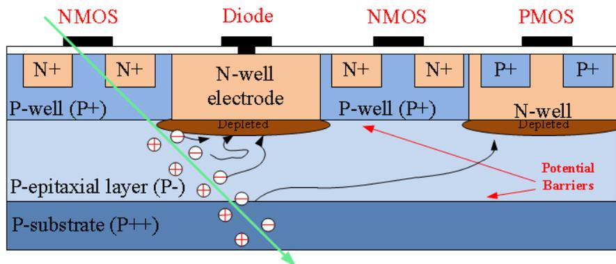
Figure 1.11: The principal of the first-generation MAPS structure.
