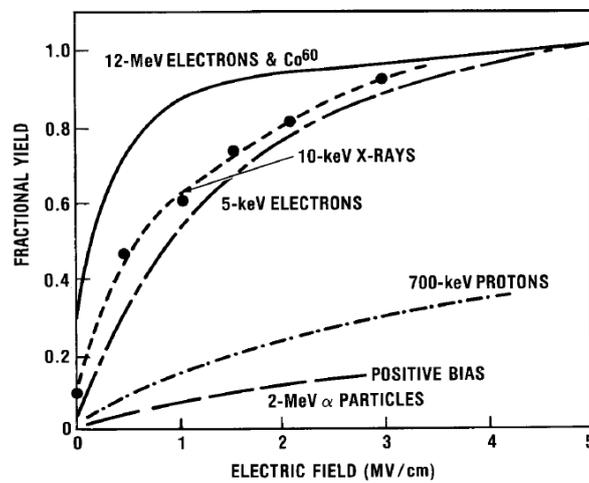
Fig. 2.16. The fractional yield of holes generated in SiO<sub>2</sub> as a function of the electric field in the material [38].
