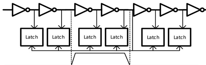
Figure 6.1. On-chip characterization of the SET pulse width.
