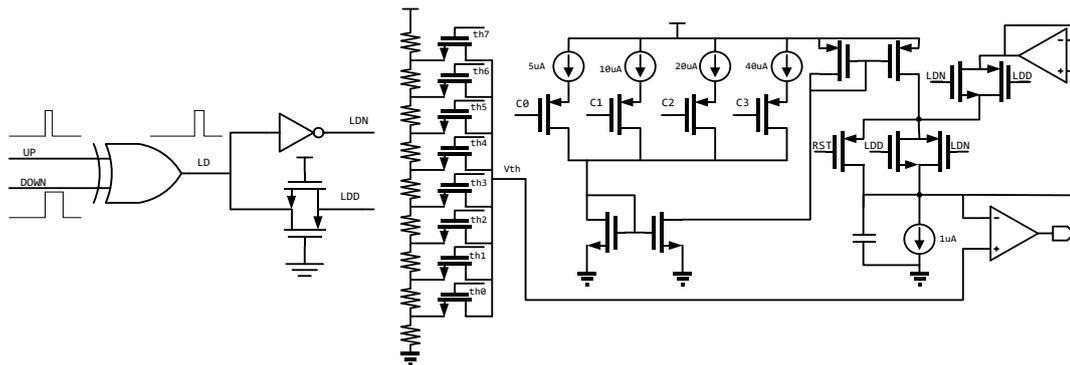
Figure 5.14 The new lock detection circuit schematic.
