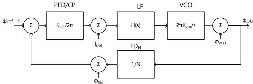
Figure 5.2 The phase-domain model of CPPLL.
