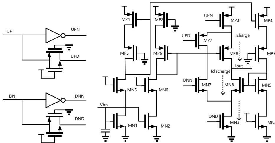
Figure 5.5 The schematic of the charge pump
