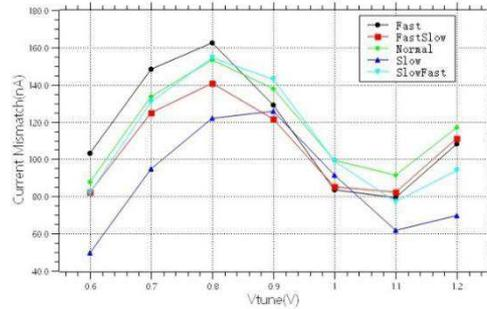
Figure 5.17. The simulation result of the current mismatch.
