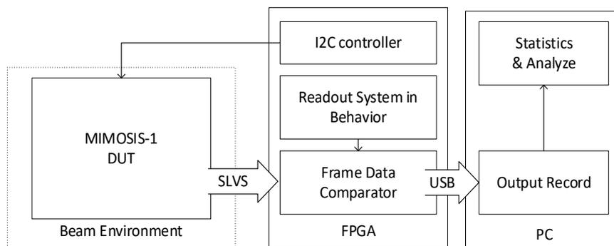
Figure 6.8. The beam test block diagram of MIMOSIS-1
