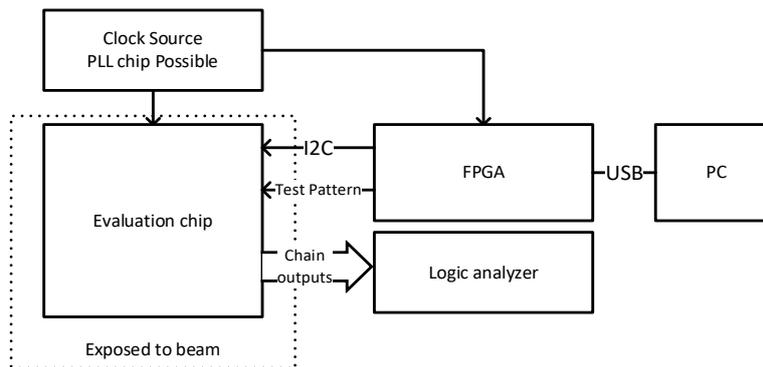
Figure 6.5. The test structure of the evaluation chip.
