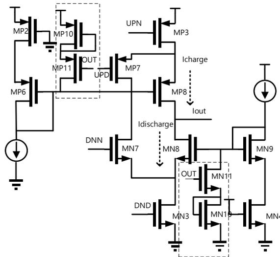
Figure 5.16. The additional feedback path of the charge pump. The dashed frame circuit helps offset the channel length modulation effect, resulting in better current matching.
