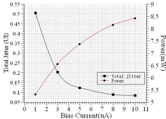
Figure 5.22. The performance of the PLL-1 with external bias. In power consumption, the configuration circuit belongs to the core part, also take into account.
