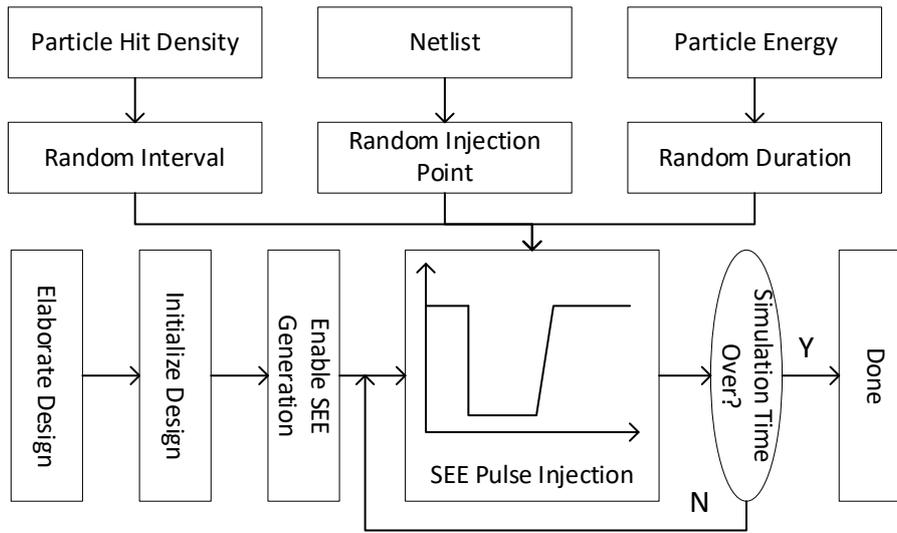
Figure 4.22. The simulation flow with SEE pulse generation.
