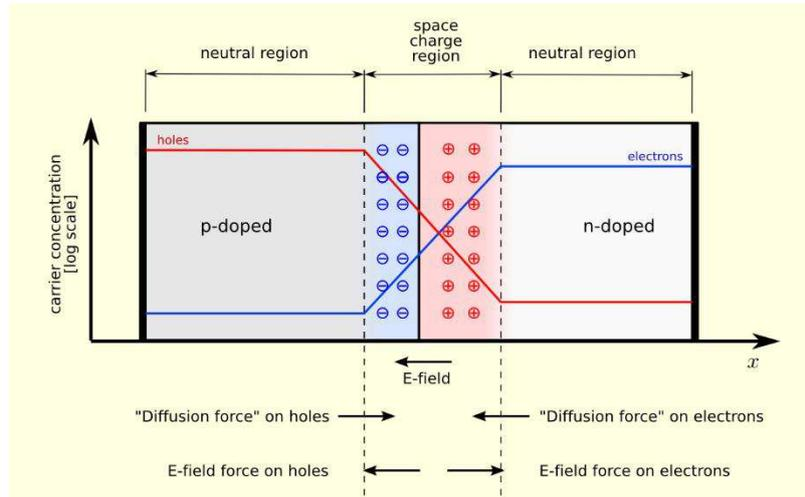
Figure 1.7. PN junction with zero bias thermal equilibrium. The electron and hole concentrations are indicated by blue and red lines, respectively. The gray area is electrically neutral. Bright red areas are positive, and bright blue areas are negative. The electric field is shown at the bottom. Electrostatic forces act on electrons and holes and their diffusion orientation [12].
