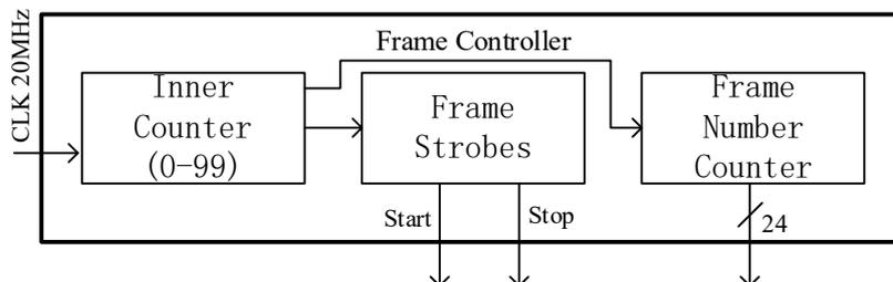
Figure 4.8. The diagram of frame controller.
