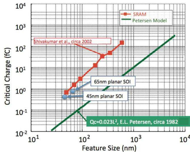
Figure 7.2. Critical charge scaling as a function of feature size. SRAM data from [6] are shown in red. The 1980's scaling model [7] is based on a second power dependence on feature size is shown in green.
