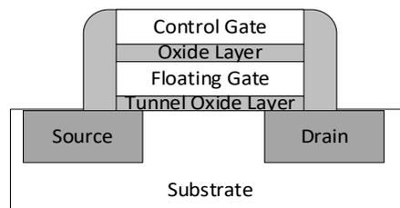
Figure 3.6. The Structure of EPROM and Flash Memory.
