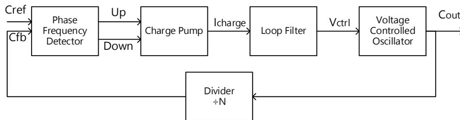
Figure 5.1 The block diagram of a typical CPPLL
