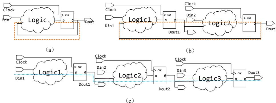
Figure 4.13. The RTL level schematic of “feedback loop registers” and flow processing registers. Part (a) and (b) have a feedback path in the data path. Part (c) is a flow processing data path.
