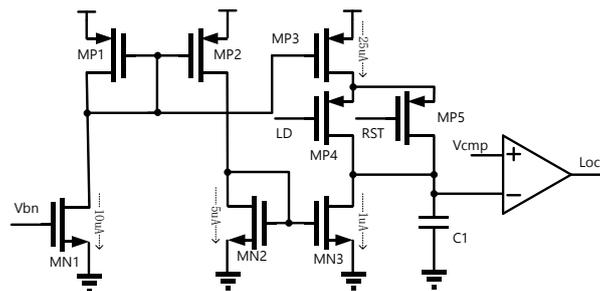
Figure 5.9. The Lock Detector circuit. The check limit of duty cycle of LD is fixed as 4%.
