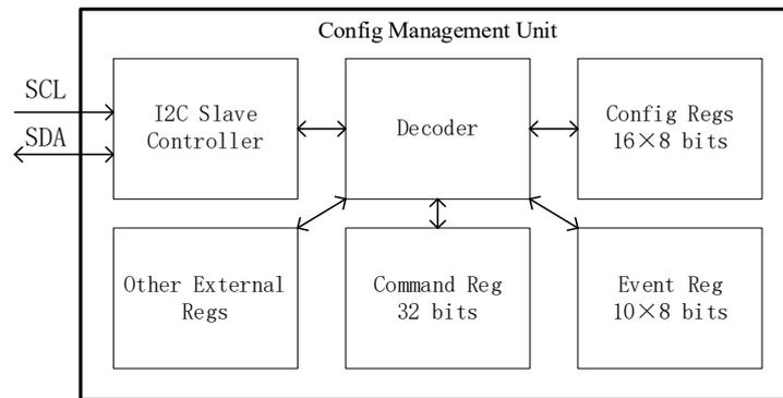
Figure 4.7. The diagram of Configuration Management Unit.
