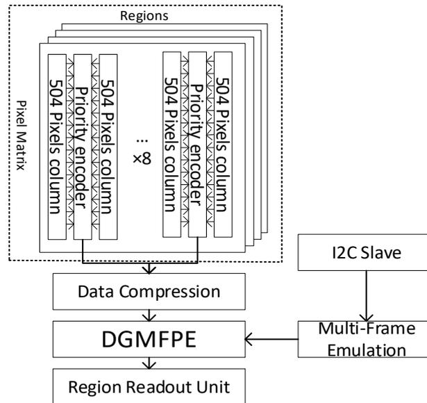
Figure 6.7. The DGMFPE module in the readout system.
