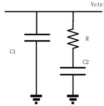
Figure 5.10. The second-order loop filter for CPPLL.
