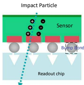
Figure 1.9 The Principal of Hybrid Pixel Sensor
