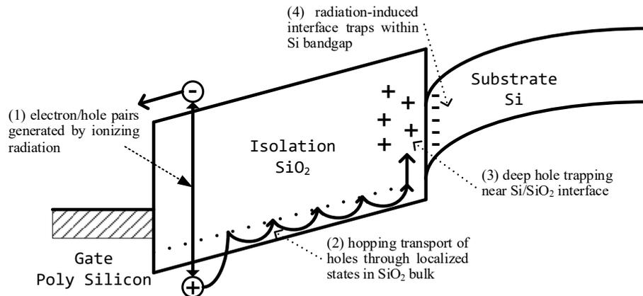
Fig. 2.15. Illustration of the main processes in TID damage [35].
