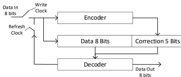
Figure 4.18. Hamming code correction protected register schematic.
