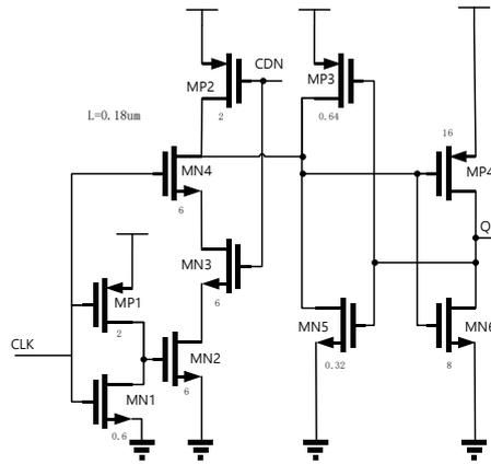
Figure 5.8 The schematic of register optimized for PFD.
