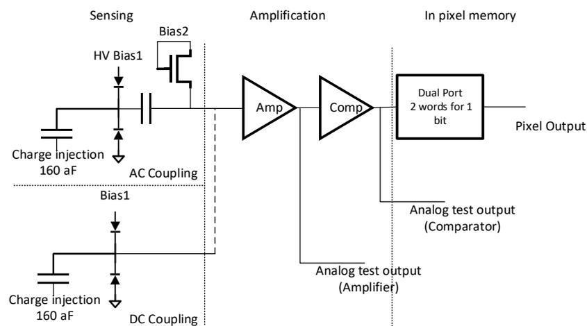
Figure 1.13 Block diagram of the pixel of MIMOSIS.
