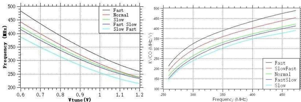
Figure 5.4 Corner simulation of output frequency and  $K_{VCO}$  versus  $V_{tune}$ .
