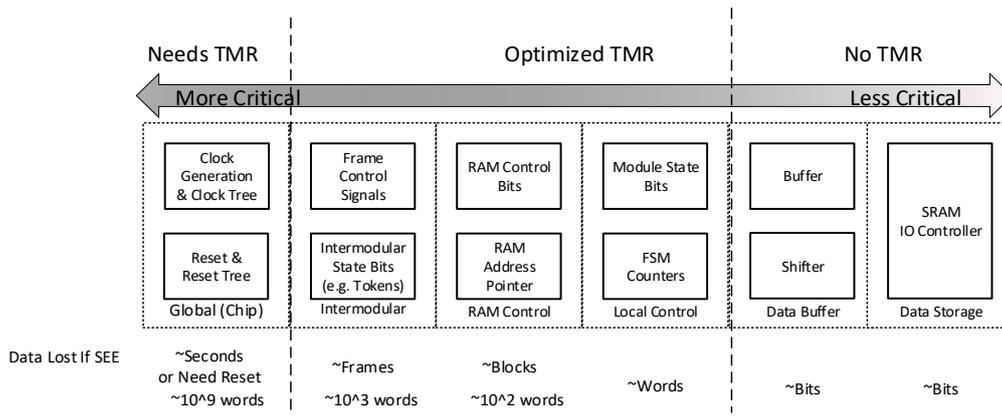
Figure 4.11. The sort of the critical level over SEE of the blocks in readout system. Registers and SRAMs are mainly concerned. Also the clock and reset circuits are involved.
