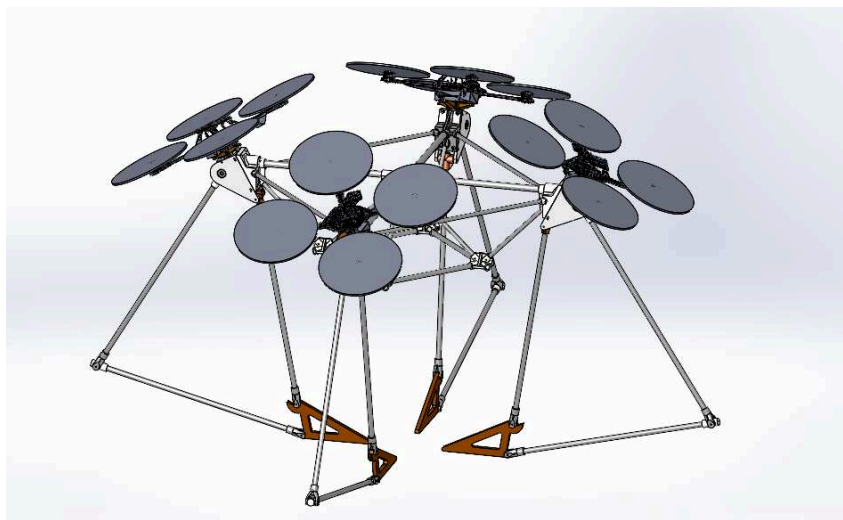
Figure 5.20 – CAD view of FG-MAQ with new structure
