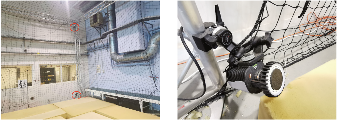
Figure 5.12 – Quadrotor arena and Motion Capture System cameras (in the red circles)
