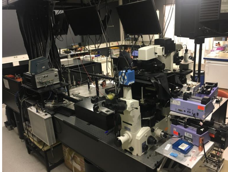
Figure 2.12. Laser and microscope setup for microfluidic NPLIN and FLIM mounted with the microfluidic system.
