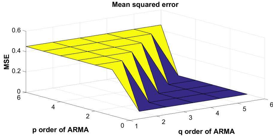
Figure 5.9 – Minimum MSE vs. orders p and q of ARIMA model.
