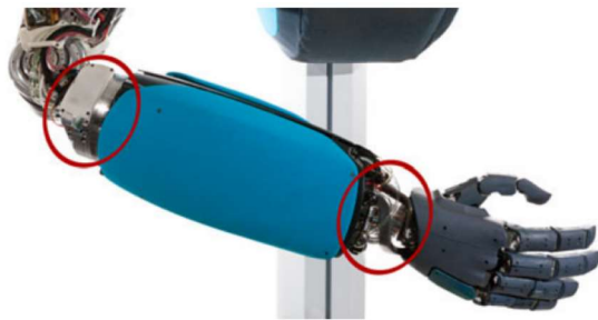
(a) Avant-bras du DLR Hand Arm System [Pet+14].
