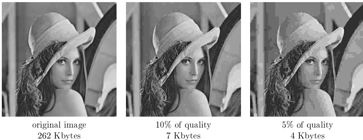
Figure 1.4: Lena (512x512 grayscale image) generated by linux batch conversion, from original (on left) to jpeg versions, by keeping 10% (middle) and 5% (right) of the quality, and reducing size of image from 163 Kbytes to 4 Kbytes
