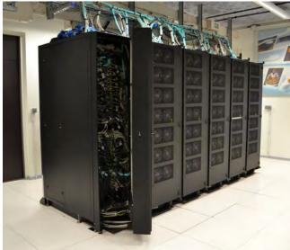
Figure 1.2: On left, a picture of the IFP Energies nouvelles supercomputer, called ENER440, at Lyon - Solaize, with details of its back (right picture) and its cooling doors equipped with cold water circuit 13 degrees.
