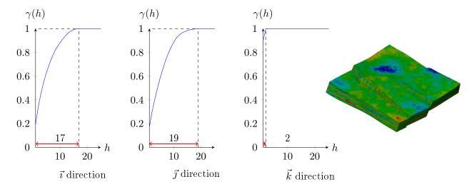
Figure 4.13: 1D variogram curves of the permeability property in the nearshore<sub>1</sub> environnement.
