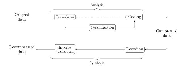
Figure 1.3: Classical compression/decompression pipeline.
