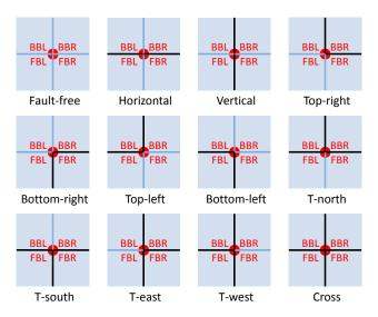
Figure 3.7: The 12 possible fault configurations (in black lines) at a given node.
