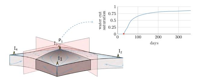
Figure 4.1: (Left) illustration of a quarter five-spot model. Blue dotted lines depict motion of water injected from corners by four wells noted  $I_i$  up to producer  $P_1$  on the top of anticline. Our model LUNDI (quarter of anticline) is highlighted in brown and limited by vertical red planes. It only considers two wells ( $I_1$  and  $P_1$ ) among five. (Top-right) water cut curve measured over a year at  $P_1$ . The red dot indicates the water breakthrough.
