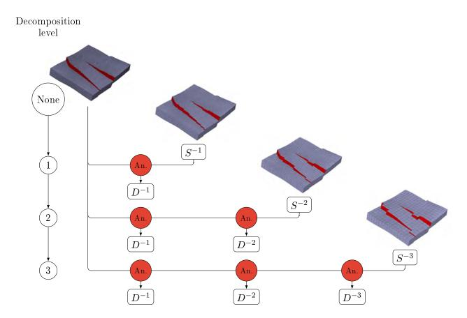
Figure 3.2: A |L|-level decomposition of a geological mesh obtained by MRA (mesh#6 from Figure 3.5). From the initial mesh (top-left), an approximated version of the initial mesh ( $S^L$ ) plus |L| sets of details ( $D^i$ ) are obtained. The number of sets of details increase with the level of decomposition |L|, but the global quantity of data remain stable.
