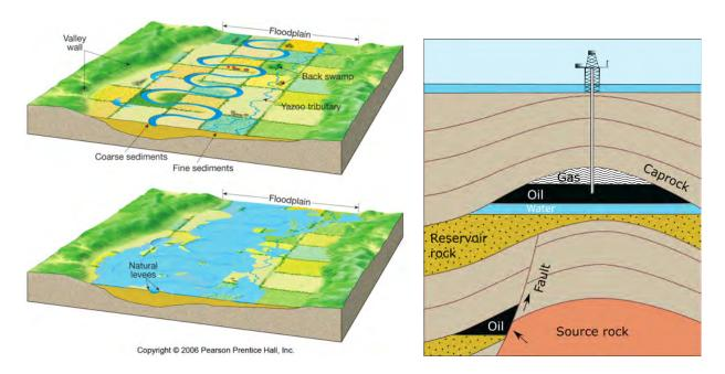
Figure 2.2: Illustration of geological structures, with fluvial deposit environment (left) and schematic geological cross section of basin, and resources localization (right).
