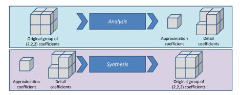
Figure 3.3: Analysis and synthesis stages for VMs.
