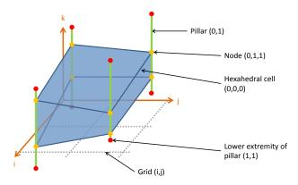
Figure 2.7: An hexahedron, according to the pillar grid structure.
