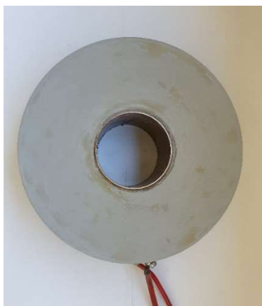
Figure 5.10: Electro-magnetic lens recuperated from a Philips CM30 transmission electron microscope (TEM) used as a solenoid
