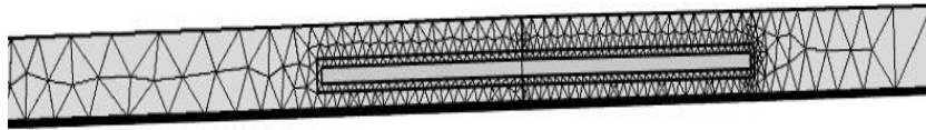
Figure A.4.5 Discretization of the computational domain in the vicinity of a filler
