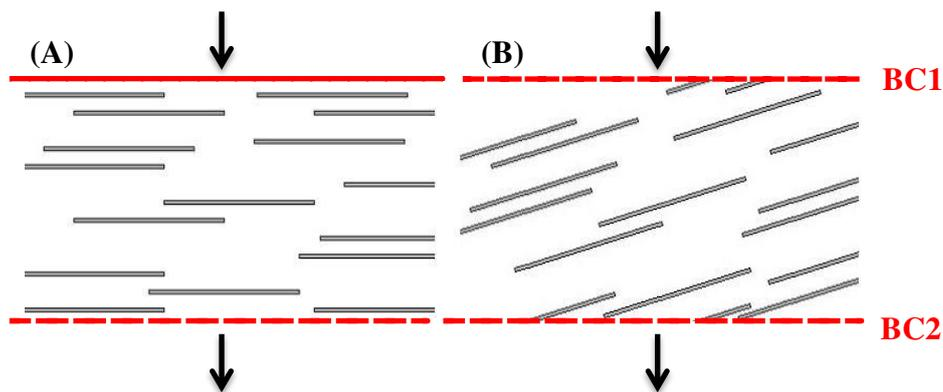
**Figure A.1.11** Fillers random dispersion in 2D systems. BC indicate boundary conditions imposed at the upper and lower faces of the system. Arrows indicate mass flux direction. (A): filler mid-plane perpendicular to mass flux direction; (B): filler mid-plane angled with respect to mass flux direction.
