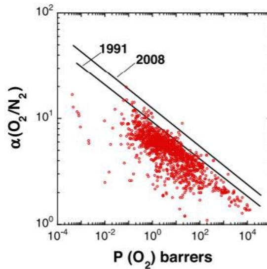
**Figure B.1.2** O<sub>2</sub>/N<sub>2</sub> upper-bound curve in polymeric membranes
