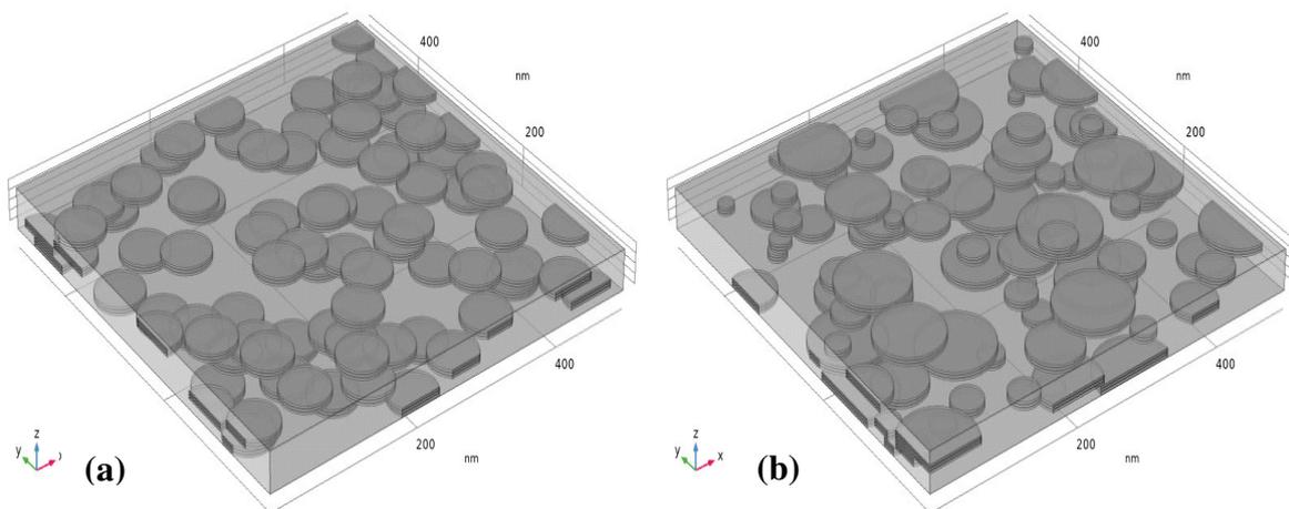
**Figure A.3.10** Example of 3D simulation domain of intercalated nanocomposites; **(a)** Monodisperse stacks **(b)** Polydisperse stacks (uniform distribution)
