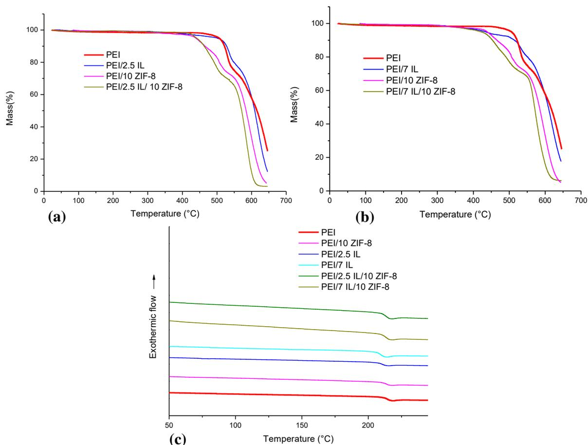
**Figure B.2.10** (a), (b) TGA and (c) DSC plots of the studied membranes
