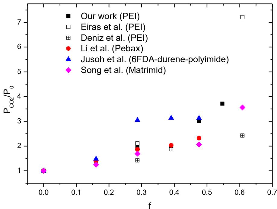
**Figure B.2.9** Comparison of the experimental data of this work with several systems based on ZIF-8 from literature (Deniz, 2012; Eiras et al., 2016; Jusoh, Yeong, Lau, & Shariff, 2016; M. Li et al., 2017; Song et al., 2012)
