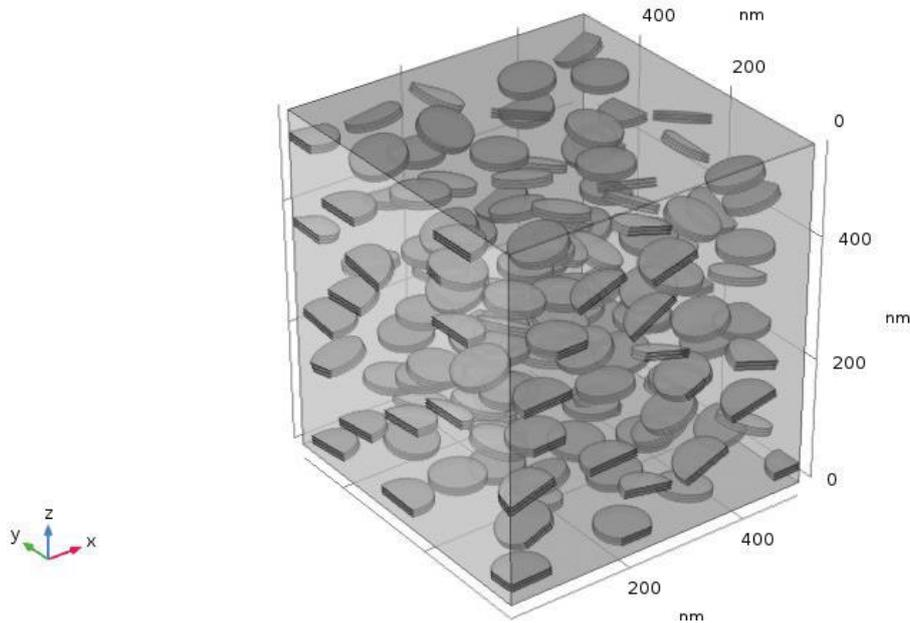
**Figure A.3.12** Geometrical model of intercalated non-oriented monodisperse system
