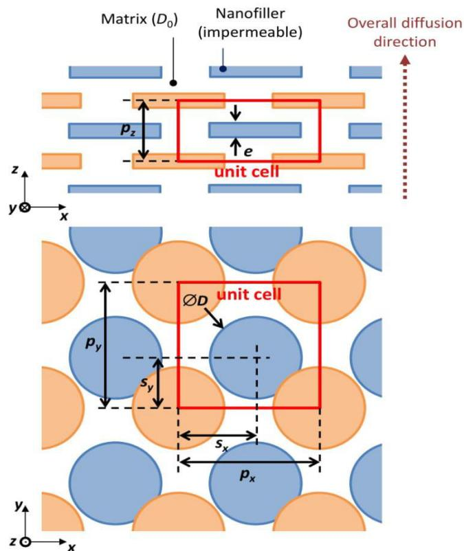
**Figure A.2.1** Geometrical model of the ordered nanocomposite and definition of the unit cell (thickness-wise and plane-wise projections)
