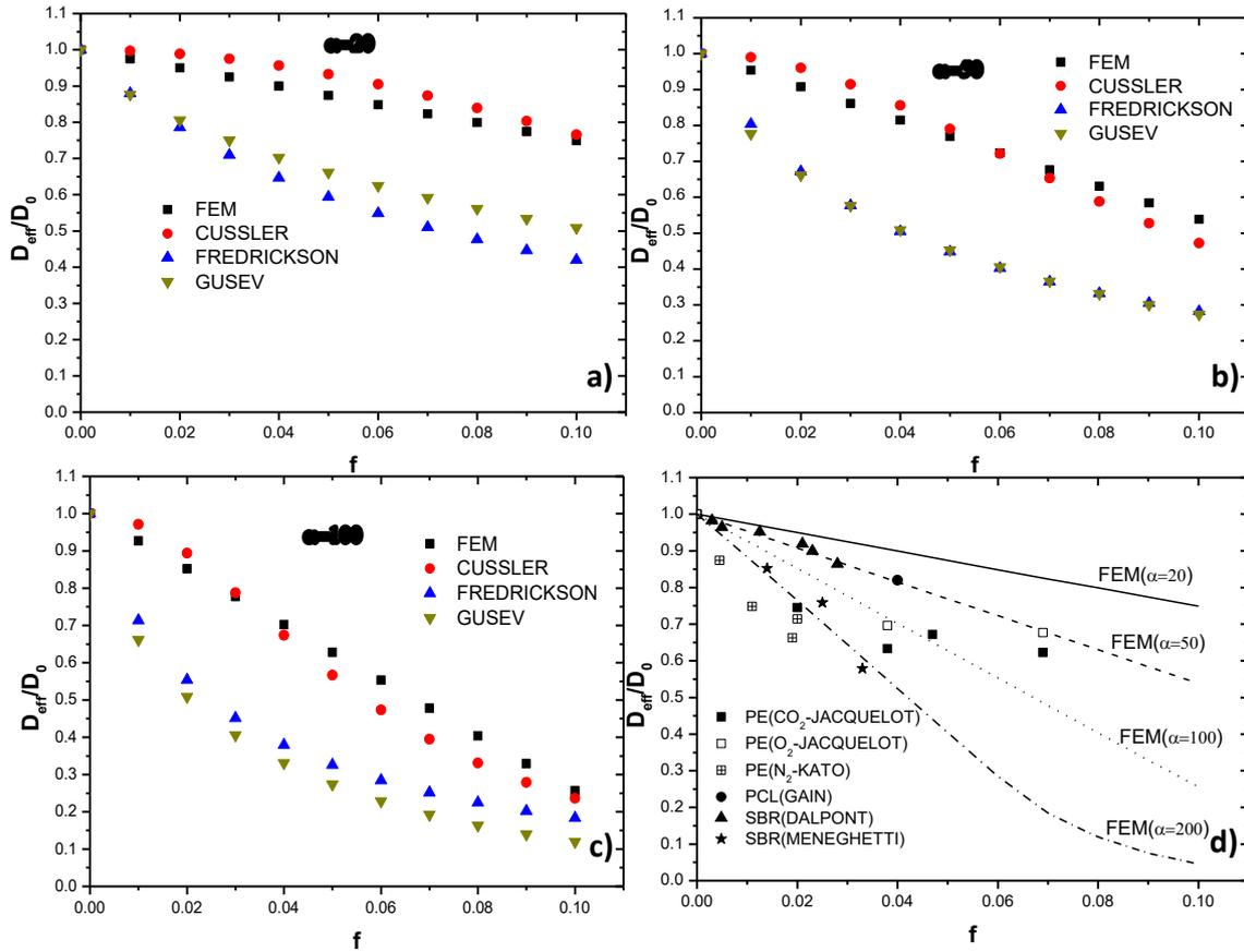
**Figure A.2.6** Comparison of numerical results to Cussler, Fredrickson and Gusev models for different values of disks aspect ratio **a)**  $\alpha=20$ , **b)**  $\alpha=50$  and **c)**  $\alpha=100$  and **d)** to literature experimental results (Dal Pont, 2011; Dal Pont et al., 2013; Gain et al., 2005; Jacquelot et al., 2006; Kato, Okamoto, Hasegawa, Tsukigase, & Usuki, 2003; Meneghetti, Shaikh, Qutubuddin, & Nazarenko, 2008)
