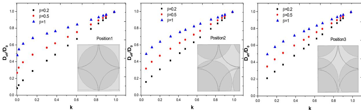
**Figure A.2.9** - Relative effective diffusivity versus the projected area ratio  $k$  for different  $\beta$  values
