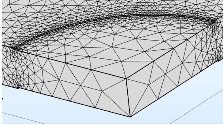
**Figure A.2.3** - Tetrahedral mesh used to discretize the computational domain
