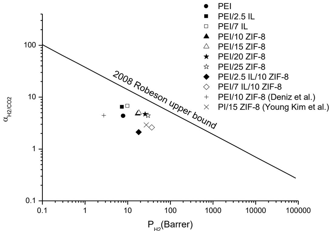
**Figure B.2.14** H<sub>2</sub>/CO<sub>2</sub> selectivity of the prepared membranes versus H<sub>2</sub> permeability compared to literature data (Deniz, 2012; E. Y. Kim et al., 2019)
