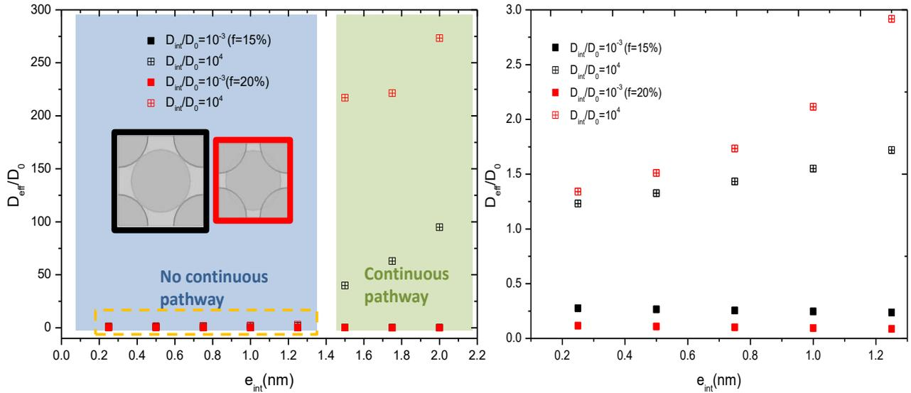
**Figure A.4.11 (a)** Relative effective diffusivity variation as a function of interphase thickness showing the presence of the continuous path **(b)** Zoom in the discontinuous pathway part showing differences in  $D_{eff}/D_0$  values
