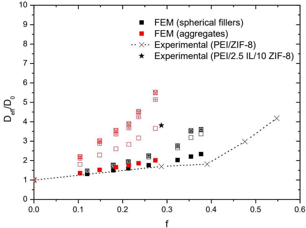
**Figure B.2.16** Comparison of the experimental relative effective diffusivity (  $\times$ : PEI/ZIF-8;  $\star$ : PEI/2.5 IL/7 ZIF-8) and numerical results obtained for several  $D_{ZIF-8}/D_0$  values: (  $\blacksquare$ : 10;  $\square$ :  $10^2$ ;  $\boxplus$ :  $10^3$ ;  $\boxtimes$ :  $10^4$  and  $\boxminus$ :  $10^5$ )
