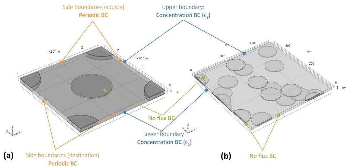
**Figure A.4.4** Representation of the RVE showing the boundary conditions: **(a)** ordered distribution; **(b)** random distribution
