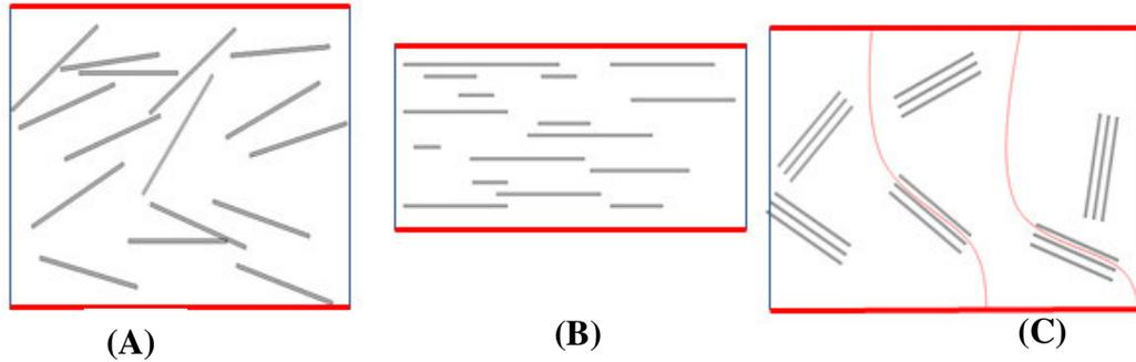
**Figure A.1.15** Fillers randomly distributed in 2D: (A) random orientation; (B) polydisperse fillers; (C) stacks of fillers (intercalated system) with diffusive flux lines. Bold red lines correspond to the inlet and outlet boundaries for mass diffusion.
