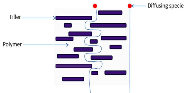
**Figure 1.2** Gas transport process through nanocomposites showing the tortuous path
