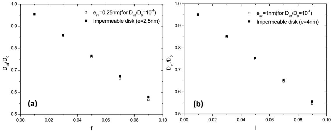
**Figure A.4.7** Comparison between the overall diffusivity for systems presenting low diffusivity interphase and fully impermeable interphase (a)  $e_{int} = 0.25 \text{ nm}$ ; (b)  $e_{int} = 1 \text{ nm}$
