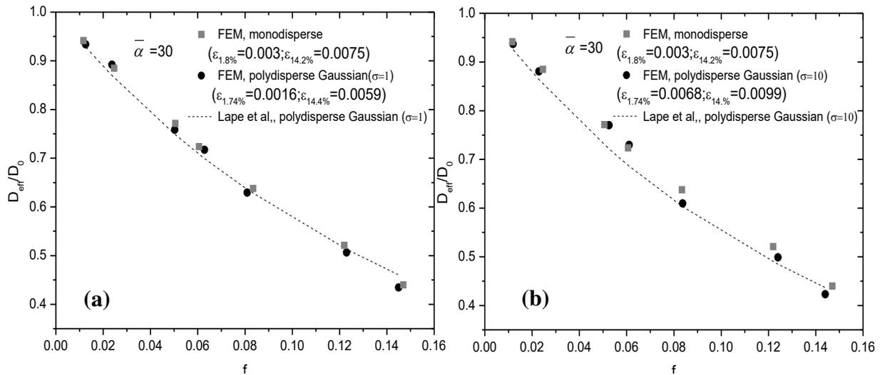
**Figure A.3.7** Relative effective diffusivity vs. filler volume fraction for monodisperse and polydisperse Gaussian systems ( $\sigma = 1$  (a) and  $\sigma = 10$  (b)): FEM predictions and Lape et al. model (Lape et al., 2004)
