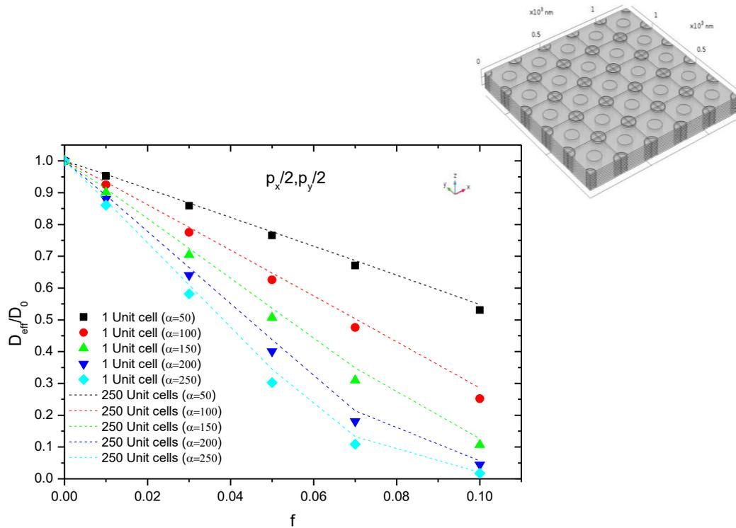
**Figure A.2.5** The effect of the number of unit cells on the overall diffusivity for different filler volume fraction and aspect ratio values
