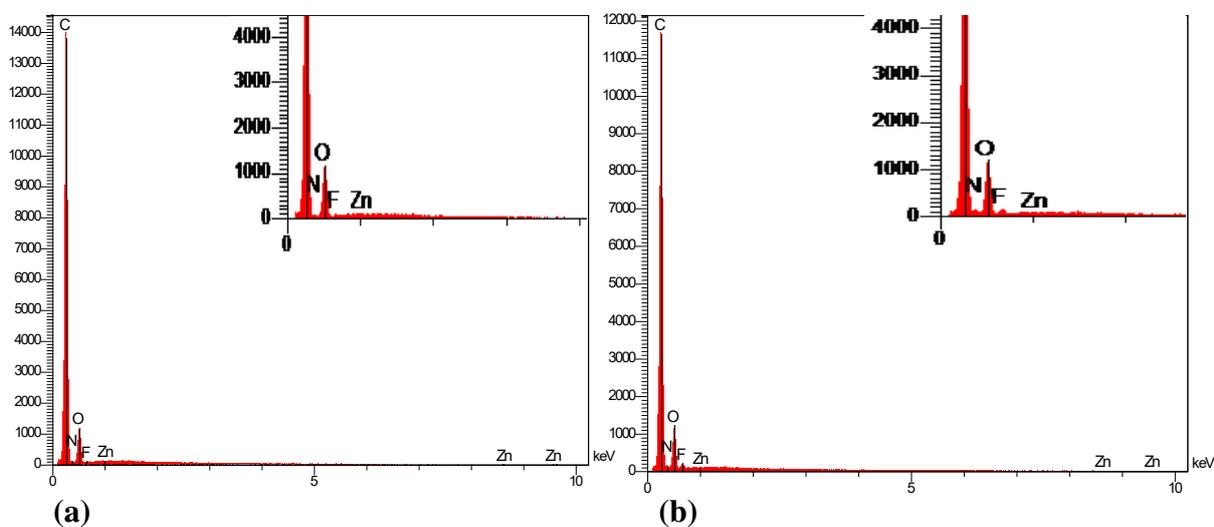
**Figure B.2.3** EDX spectra of (a) PEI matrix and (b) IL
