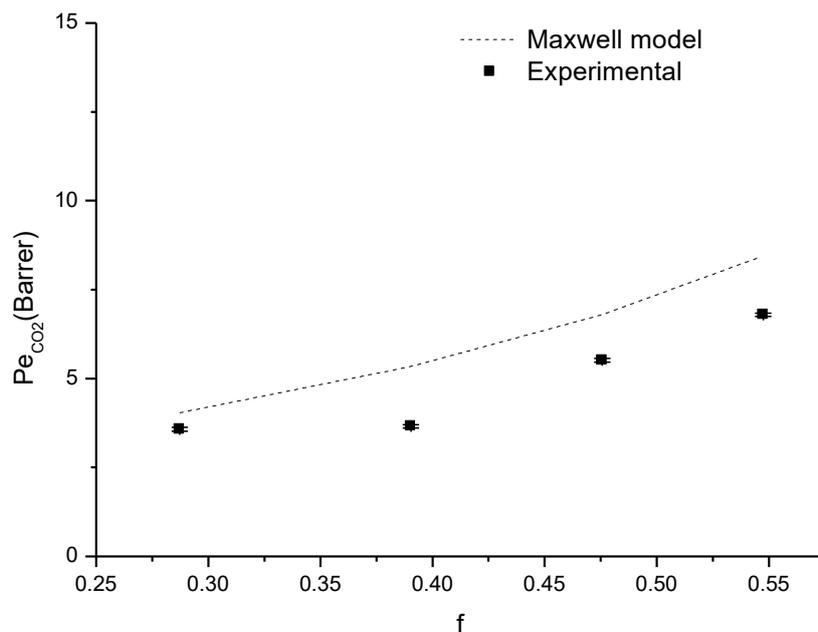
**Figure B.2.8** Comparison between Maxwell model and experimental CO<sub>2</sub> permeability coefficients for the studied membranes
