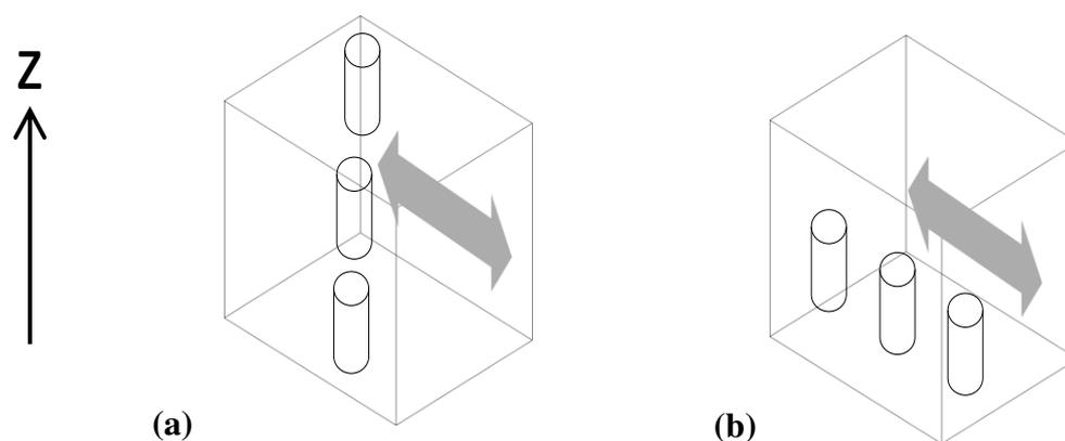
**Figure B.1.6** The geometry used in Wang et al. work (a) fillers parallel to z-axis (mass flux direction) (b) fillers normal to z-axis (mass flux direction) (T. P. Wang & Kang, 2015)
