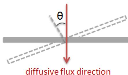
**Figure A.1.12** Angle of orientation defined in the cited models
