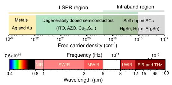
Figure II.17 The relation between the absorption spectra and the doping magnitude. The lower panel shows a spectrum from visible to THz, and the upper panel indicates the corresponding carrier density required for such absorptions, either in the form of LSPR when the materials are highly doped or in the form of intraband transition when the material is in a confined regime with margin doping.
