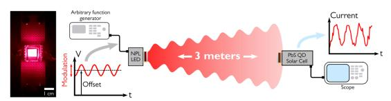
Figure III.17 Schematic graph of a LiFi-like communication setup. In the setup, the large LED is driven under a constant bias, on top of which a modulated signal is added. The signal is then collected by a PbS nanocrystal based solar cell used as a broad band detector from a distance.
