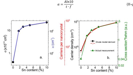
Figure II.20 (a) The measured absorption coefficient  $\alpha$  and the corresponding absorption cross section  $\sigma$  as a function of Sn content.(b)The estimated carrier density and the number of carriers per nanocrystal from Dude model, in comparison with the production of and LSPR fwhm and absorption cross section, as a function of Sn content.
