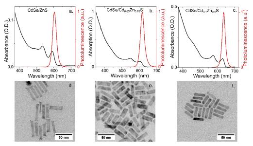
Figure III.6 Absorption and photoluminescence spectra and TEM images of CdSe/ZnS (a) and (d), CdSe/Cd<sub>0.05</sub>Zn<sub>0.95</sub>S (b) and (e), and CdSe/Cd<sub>0.1</sub>Zn<sub>0.9</sub>S (c) and (f) core/shell NPLs.
