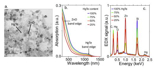
Figure III.33 (a) TEM image of HgTe(25%)/ZnO mixture. (b) Absorption spectra of mixture made of HgTe/ZnO nanocrystals with various HgTe content. (c) Energy dispersive X-ray spectroscopy spectrum relative to mixture made of HgTe/ZnO nanocrystals with various HgTe content.
