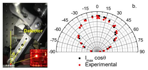
Figure III.10 (a) Scheme of the setup used to measure the angular dependence of EL, in which the angle  $\theta$  is the angle between the detector and the normal of LED plane. In the inset is the working pixel. (b) Comparison between the experimental EL intensity and a cosine dependence of EL intensity for the light emitted by the NPL based LED.
