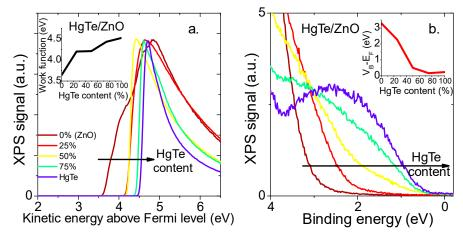
Figure III.35 (a) Photoemission spectra relative to the secondary electron cut-off for ZnO/HgTe thin films with various HgTe content. Inset: the change of work function with the HgTe content in the mix, (b) Low binding energy part of the photoemission spectra, relative to the valence band of ZnO/HgTe with various HgTe content. Inset: the energy difference between valence band and the Fermi level as a function of the HgTe content in a ZnO/HgTe mixture.
