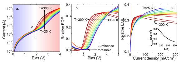
Figure III.15 (a) Current as a function of bias under various temperatures for an LED device based on  $CdSe/Cd_{0.05}Zn_{0.95}S$  core/shell NPLs (b) Uncalibrated EQE as a function of the applied bias under various temperatures. (c) Uncalibrated EQE as a function of the driving current density under different temperatures. The curves are collected every 25 K from 300 K to 25K.
