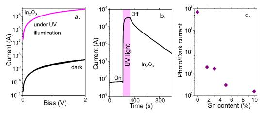
Figure II.25 (a) I-V curve of  $In_2O_3$  nanoparticles under dark condition and under UV illumination. (b) Current as a function of time while a thin film  $In_2O_3$  nanoparticle is exposed to a pulse of UV light. (c) Current modulation (ratio of the photocurrent over the dark current) as function of the Sn content of an ITO thin film exposed to a short illumination of UV light.
