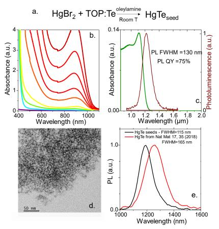
Figure III.43 (a) Chemical reaction conducted to obtain small HgTe seeds. (b) UV-vis absorption spectra for a mixture of HgBr<sub>2</sub> and TOP:Te in oleylamine at room temperature, leading to HgTe seeds. (c) Absorption and PL spectra of the quenched HgTe seeds. (d) TEM image of the HgTe seeds. (e) Comparison of PL spectrum between HgTe seeds and the HgTe synthesized using the procedure from Geiregat *et. al.* <sup>265</sup>
