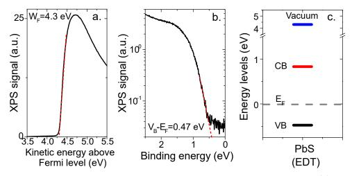
Figure III.30 Photoemission spectra relative to the secondary electron cut-off (a) and relative to the valence band (b) of PbS nanocrystal film with an excitonic peak at 960 nm and capped with EDT. (c) Proposed electronic spectrum of the EDT-capped PbS nanocrystal array with respect to vacuum level.
