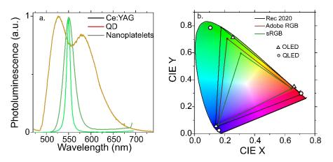
Figure III.1 PL spectra of traditional phosphor (Ce:YAG), QDs and NPLs, with nanocrystals showing much narrower linewidth. (b) CIE 1930 chromatograph of different display gamut and the gamut that can be achieved by organic LEDs and quantum dot LEDs.
