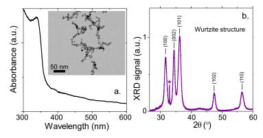
Figure III.24 (a) Absorption spectrum of ZnO nanocrystals. In the inset is a corresponding TEM image. (b) X-ray diffraction pattern of ZnO nanocrystals which shows a wurtzite structure. The peak marked with \* corresponds to Si substrate uner the sample.
