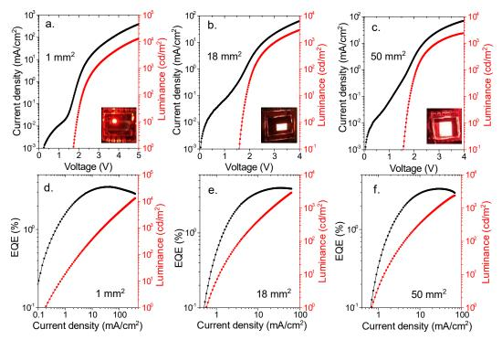
Figure III.18 Current density and luminance as a function of bias for the pixels of  $1 \text{ mm}^2$  (a), 18 mm<sup>2</sup> (b) and 50 mm<sup>2</sup> (c). EQE and luminance as a function of current density for the pixels of  $1 \text{ mm}^2$  (d), 18 mm<sup>2</sup> (e) and 50 mm<sup>2</sup> (f). In the inset are the working devices of different size corresponding to the curves.
