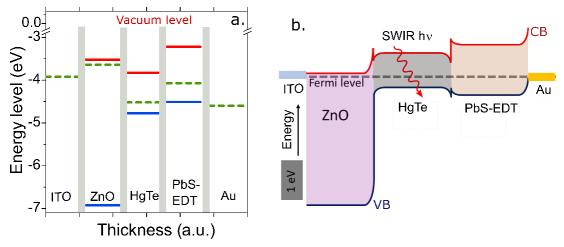
Figure III.32 (a) Band alignment of the different layers involved in the ITO/ZnO/HgTe/PbS/Au diode, with o eV corresponding to the vacuum level, the red line to the conduction band, the blue line to the valence band, and the green dashed line representing the Fermi level. (b) Schematic illustration of band bending in the LED device without applying a bias.
