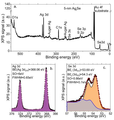
Figure II.10 (a) The XPS overview of a film made from  $5 \text{ nm } Ag_2Se$  nanocrystals. (b) Ag 3d core level of a film made from  $5 \text{ nm } Ag_2Se$  nanocrystals. (c) Se 3d core level of a film made from  $5 \text{ nm } Ag_2Se$  nanocrystals.
