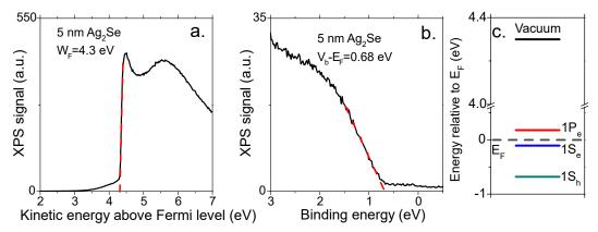
Figure II.7 (a) Photoemission signals of secondary electron cut-off for a film made of 5 nm  $Ag_2Se$  nanocrystals. The determined work function is 4.3 eV. (b) Photoemission signals associated with the valence band for a film made of 5 nm  $Ag_2Se$  nanocrystals. The Fermi level is 0.68 eV above the valence band. (c) A proposed electronic spectrum in the absolute energy scale for 5 nm  $Ag_2Se$  nanocrystals, with a Fermi level in the conduction band.
