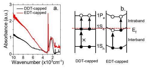
Figure II.11 (a) FTIR spectra of 5 nm Ag<sub>2</sub>Se capped with DDT and EDT ligands. (b) A scheme describing the band bending and doping conditions of the Ag<sub>2</sub>Se nanocrystals capped with DDT and EDT.
