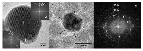
Figure II.9 The identification of  $Ag^{\circ}$  from the TEM of  $Ag_2Se$  nanocrystals. (a) The TEM image of the 28 nm nanocrystals. FFT of the area 1 (inset to the down left) and the area 2 (inset to the up right) revealing a crystal structure of Ag metal and tetragonal  $Ag_2Se$ . (b) TEM image of  $Ag_2Se$  nanocrystal in which five arrows indicates five twins. (c) The corresponding FFT of (b), indexed with FCC crystal structure of silver.
