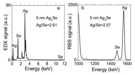
Figure II.8 (a) EDX signal of a film made of 5 nm  $Ag_2Se$  nanocrystals, revealing a ratio of Ag/Se=2.61. (b) RBS signal is associated with a film made of 5 nm  $Ag_2Se$  nanocrystals, leading to Ag/Se=2.57.
