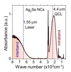
Figure II.14 FTIR of 5 nm Ag<sub>2</sub>Se nanocrystals, with its interband and intraband transitions excited by 1.55  $\mu$ m laser diode (indicated by blue dash line) and 4.4  $\mu$ m quantum cascade laser (indicated by red dash line), respectively.
