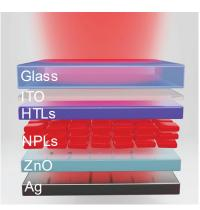
Figure III.4 Schematic diagram of a LED made of glass/ITO/HTLs (PEDOT:PSS/PolyTPD/PVK)/ CdSe/CdZnS core/shell NPLs/ZnO/Ag, with ITO and Ag as anode and cathode, respectively.<sup>100</sup>
