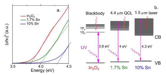
Figure II.24 (a) Tauc-plot of UV-Vis spectra of ITO nanocrystals, with the intersection of the liner region with x-axis as the optical bandgap. (b) Band diagram of undoped  $In_2O_3$ , 1.7% Sn and 10 % Sn doped ITO nanocrystals. UV is used to excite the band edges of the nanocrystals, while blackbody, 4.4 µm quantum cascade laser and 1.5 µm laser diodes are used to excite the infrared transition of  $In_2O_3$ , LSPR transition of 1.7% Sn and 10 % Sn doped ITO nanocrystals.
