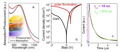
Figure III.19 (a) Absorption spectrum of the PbS nanocrystals and photocurrent spectrum of the solar cell based on the PbS nanocrystals. In the inset is a scheme of the solar cell structure. (b) I-V curves in the dark and under illumination (940 nm laser source with 56 mW.cm<sup>-2</sup>) at room temperature. (c) Time response of the PbS nanocrystal based solar cell to a 1 ns pulse of laser at 355 nm. Turn-on time is around 10 ns while turn-off is around 1 µs.
