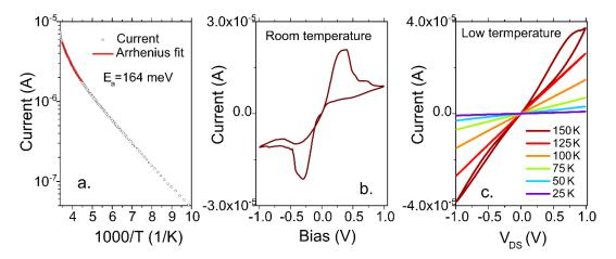
Figure II.13 (a) Variation of dark current with temperature of a device based on EDT-capped Ag<sub>2</sub>Se. (b) I-V curve of Ag<sub>2</sub>Se nanocrystal-based device at room temperature showing large hysteresis and nonlinear feature. (c) I-V curve at low temperatures below 175 K, showing an ohmic feature and no hysteresis.
