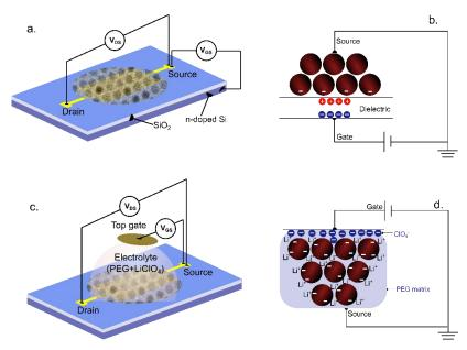
Figure I.8 (a) Scheme of a conventional back gate FET with  $SiO_2$  as dielectric and a heavily doped Si as gate electrode. (b) The gate effect induced in a nanocrystal film when  $V_{GS}$  above 0 V. (c) Scheme of an electrolyte top gate FET. (d) Gate effect induced in an electrolyte gated FET when  $V_{GS}$  above 0 V.
