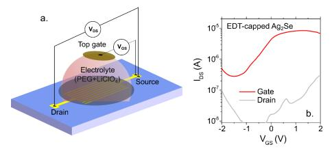
Figure II.12 (a) Scheme of electrolyte gated FET. (b) The transfer curve of EDT-capped  $Ag_2Se$  nanocrystals, with a constant drain-source voltage of 20 mV.
