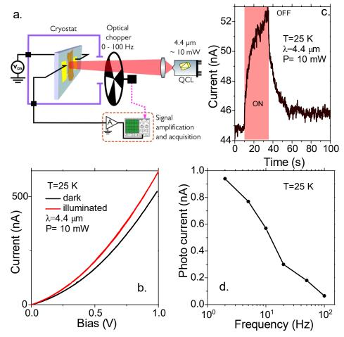
Figure II.16 (a) Scheme of the experiment setup reprinted from reference<sup>102</sup>. A 4.4  $\mu$ m QCL is aligned to illuminate the photoconductive device enclosed in a cryostat. (b) I-V curves of Ag<sub>2</sub>Se nanocrystal-based device in the dark and under illumination. (c) Current as a function of time while QCL is turned on and off. (d) Photocurrent as a function of chopping frequency.
