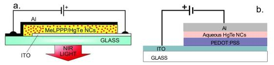
Figure III.22 (a) An infrared LED structure based on a blend of conjugated polymer (MeLPPP) and HgTe nanocrystals. The figure is adapted from <sup>174</sup>. (b) An infrared LED structure with HgTe nanocrystals as emitting layer and PEDOT:PSS transport layer.<sup>252</sup>
