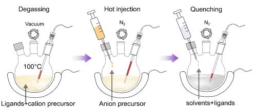
Figure I.3 Typical hot injection synthesis of colloidal nanocrystals including degassing of solvents and precursors, hot injection in an inert atmosphere and the quenching of reaction.
