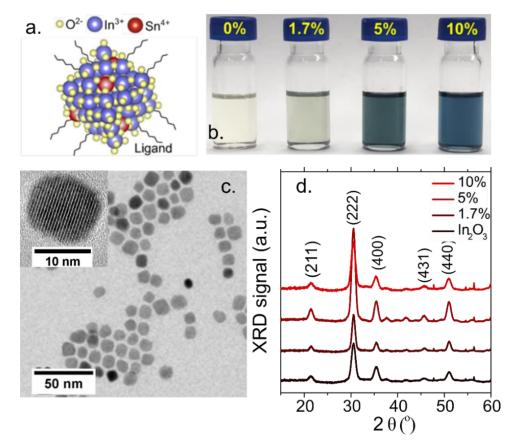
Figure II.18 (a) Scheme of a colloidal ITO nanocrystal with an ITO core surrounded by organic ligands. (b) Image of ITO nanocrystals dispersed in CHCl<sub>3</sub> with various levels of Sn content. (c) TEM image of the 1.7% Sn ITO nanocrystals. In the inset is a corresponding high-resolution TEM image. (d) XRD patterns of the synthesized ITO nanocrystals of different doping levels showing an identical bixbyite structure.
