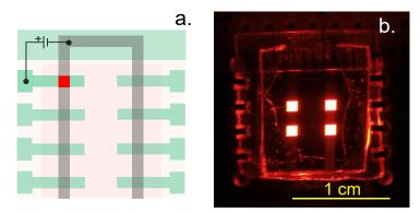
Figure III.8 (a)Scheme of the LED device where the red square represents a working pixel when applied with a forward bias. The gray "U" shape pattern represents the Ag electrode deposited under a shadow mask. (b) A working LED based on  $CdSe/Cd_{0.05}Zn_{0.95}S$  core/shell NPLs with 4 pixels (1 mm<sup>2</sup>) driven under the forward bias.
