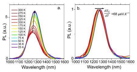
Figure III.28 PL (a) and normalized PL (b) spectra for a film made of HgTe nanocrystals at different temperatures.
