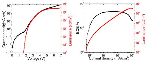
Figure III.14 (a) Current density and luminance as a function of bias. (b) EQE and luminance as a function of current density for the LED with  $CdSe/Cd_{0.05}Zn_{0.05}S$  NPLs as emitting layer.
