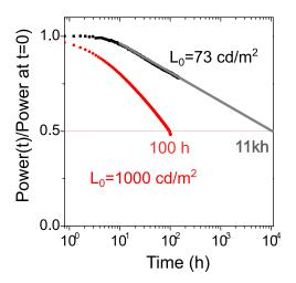
Figure III.13 The luminance variation with time at the intial luminance of  $73 \text{ cd/m}^2$  (black curve) and 1000 cd/m<sup>2</sup>(red curve).
