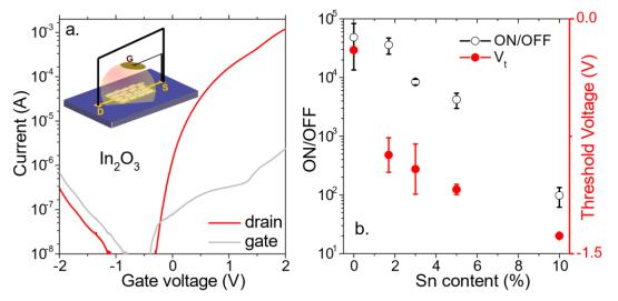
Figure II.21 (a) Transfer curve (drain and gate current as a function of the applied gate voltage) for a transistor whose channel is made of  $In_2O_3$  nanocrystals. In the inset is a scheme of an electrolyte gated transistor. (b) ON/OFF ratio and threshold voltage as a function of Sn content for transistors made of ITO nanocrystals.
