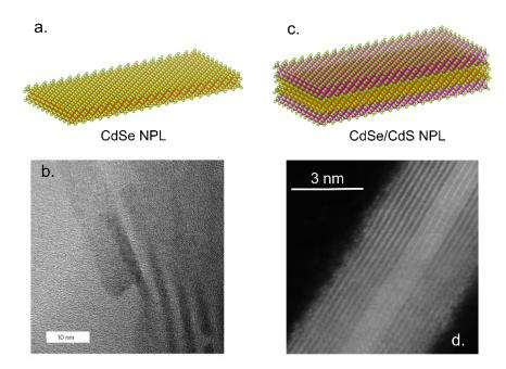
Figure I.6 Scheme of a core-only CdSe NPL (a) and a corresponding TEM (b), adapted from the reference<sup>4</sup>. Scheme of a CdSe/CdS core/shell NPL (c) and a corresponding TEM image of CdSe/CdS core/shell NPL demonstrating atomic resolution (d), TEM adapted from the reference. <sup>36</sup>
