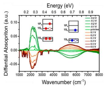
Figure II.6 Differential absorption spectra of Ag<sub>2</sub>Se nanocrystals with different electrochemical potentials: the green curve indicates the oxidation of the system while the red curve the reduction of the system. Reproduced with permission from form reference<sup>93</sup>. Copyright (2018) American Chemical Society.
