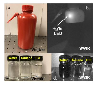
Figure III.42 Visible (a) and SWIR (b) image of a PET washing bottle with water in it. For all SWIR images, only the HgTe LED is used as light source (i.e. no visible light contribution).Visible (c) and SWIR (d) image of vials containing different solvent (water, toluene, tetrachroloethylene: TCE).
