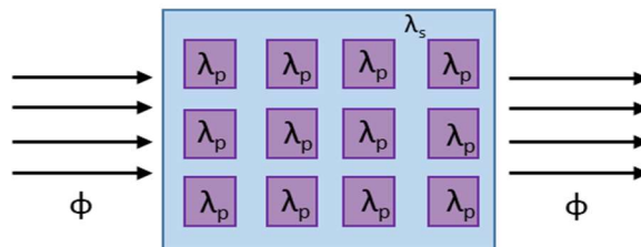
Figure 1-11: Schematic of Russell model ( \Phi = heat flow).
