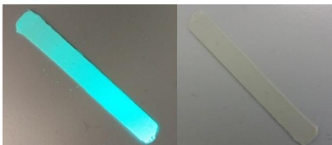
Figure 2.17: *Photographs of an EML sample under a 365 nm UV-light (left) and natural light (right). Sample dimensions: 70 mm x 10 mm x 0.7 mm*
