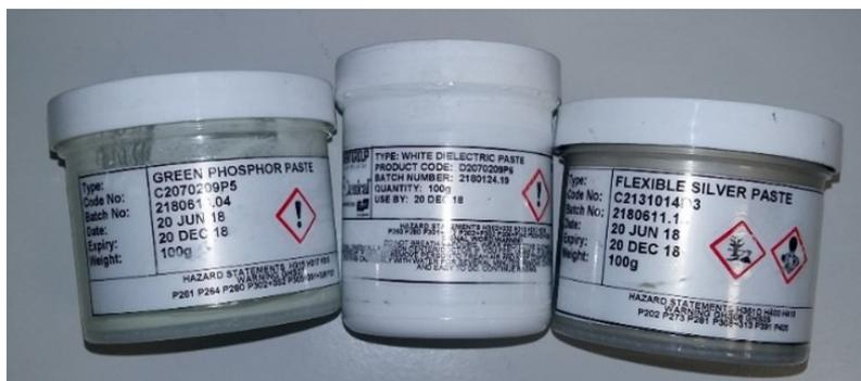
Figure 2.1: *Gwent Group electro luminescent kit. From left to right: green phosphor paste, dielectric paste, silver paste*
