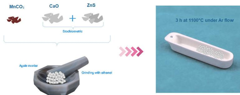
Figure 3.18: *Synthesis of  $\text{CaZnOS:Mn}$  by solid state reaction.*
