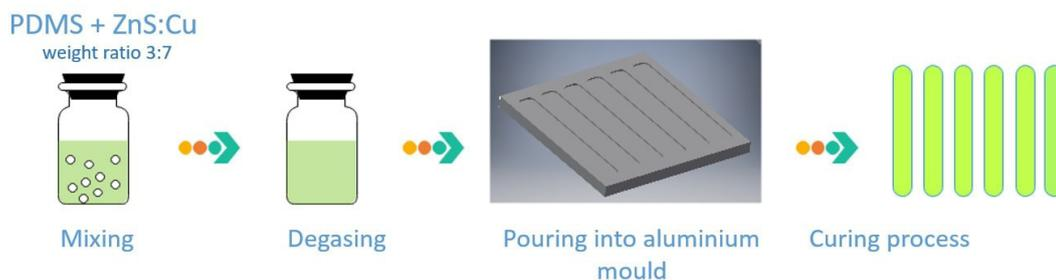
Figure 2.16: *Steps of sample making. From left to right: mixing the ZnS:Cu particles and the PDMS, degasing the sample, shaping the samples by pouring the mixture into a mould, and curing at room temperature.*
