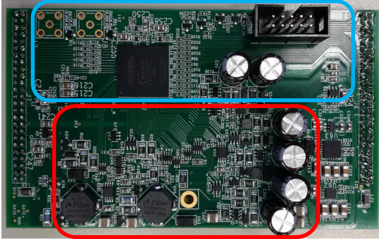
Fig. 3-6. CMUT control and supply board picture: high voltage supplies circuits (red) and control circuits (light blue).
