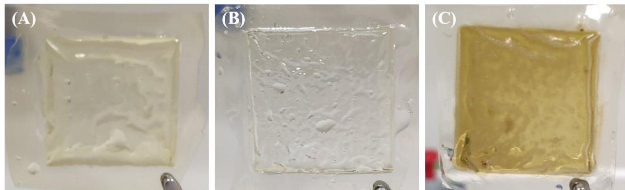
Figure 6: Photographs of membranes after the cell cycling tests. The protruding square is the tested area directly in contact with the electrodes and the electrolyte solutions: (A) M1, (B) M2 and (C) M3.
