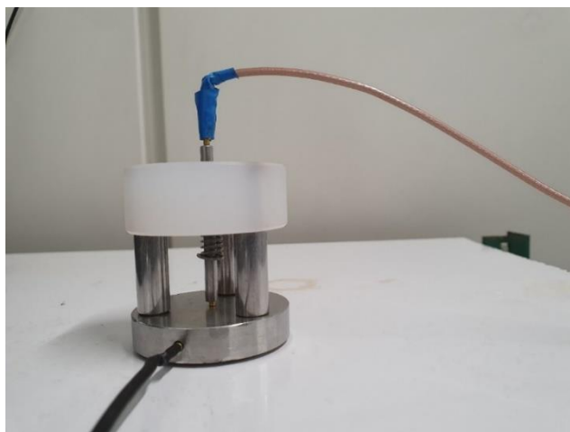
Figure 2: homemade membranes ion conductivity measuring cell.
