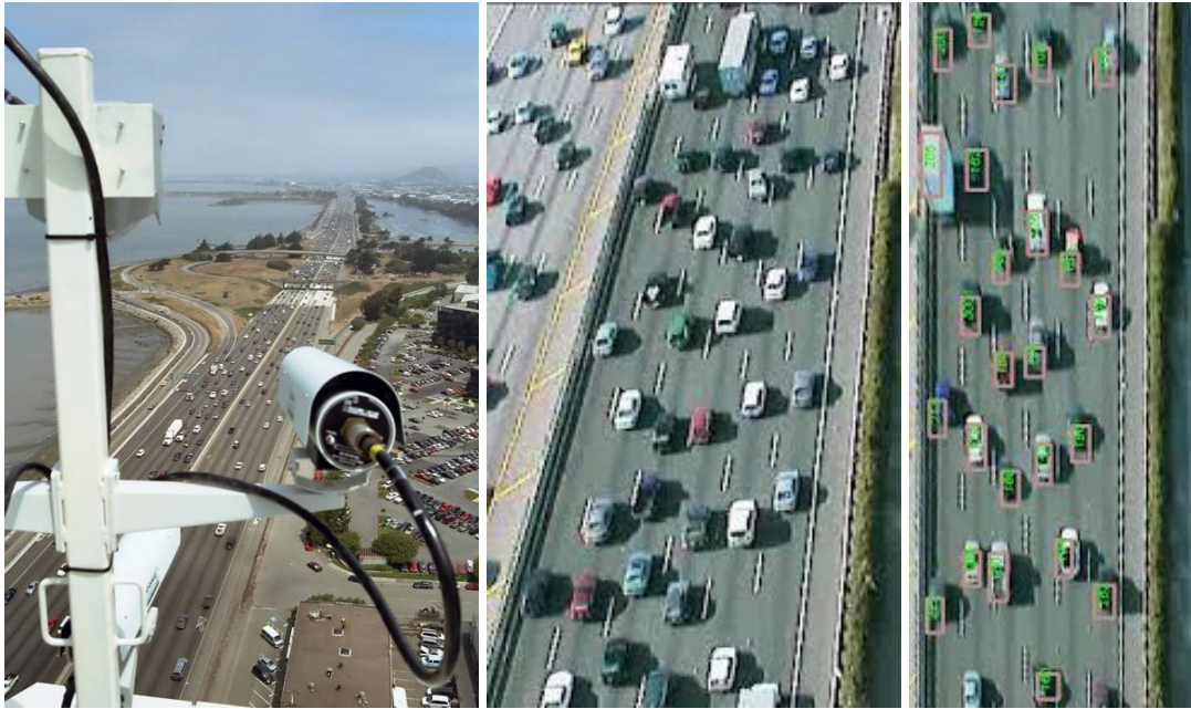
Figure 1.2: Recording system, sub-sections of the raw and processed samples for the NGSIM I-80 dataset. (source: [CH07])
