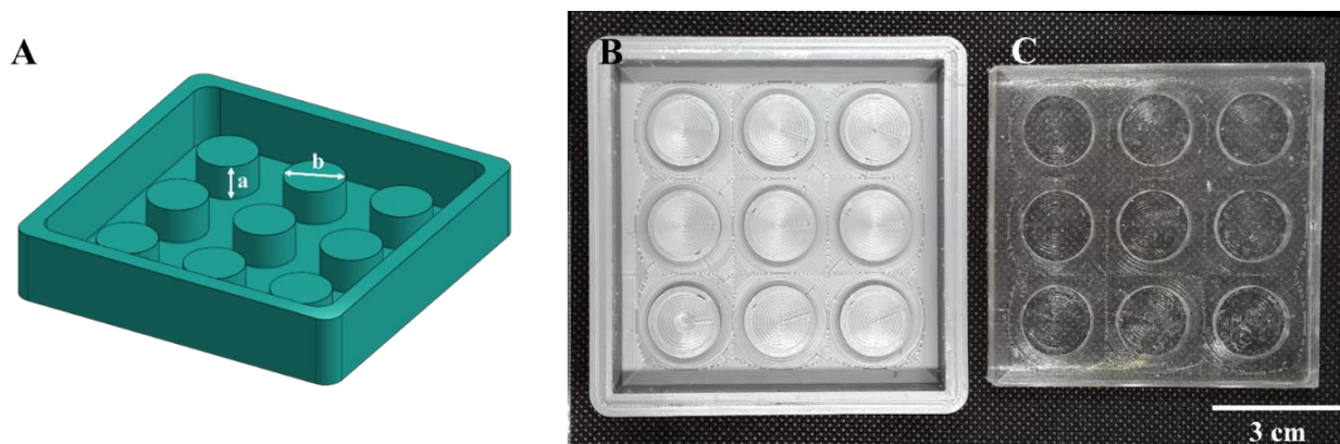
Figure A.3. CAD design (A) and PLA 3D printed (B) image of negative mold. PDMS mold (C) used for hydrogel preparation.
